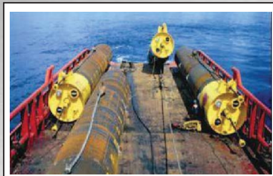
Suction type anchors.
