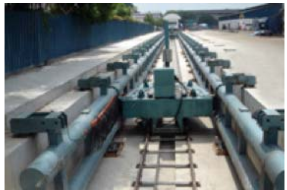
200 ton x 22.5 m Horizontal Tension tester
