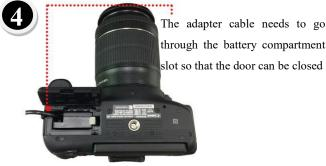
Insert the DC coupler in the battery compartment of the digital camera until it locks in place. In order to do so you need to open the battery cover first
