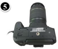
If the camera has DC cord hole cover – open it and install the cord. Close the battery cover. Now you can turn ON your Digital Camera / Camcorder
