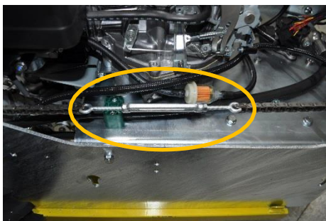
Fig. 19 - Tensioning/loosening the roller chain
