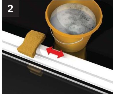
2 Grease marks, dirt and mastic spillage may be removed using soapy water.
