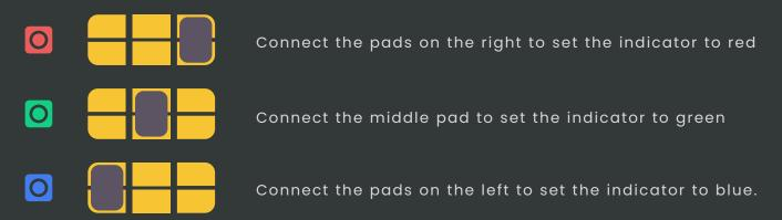
If you wish to reselect the color, use a soldering iron to remove the solder from the pads and then reconnect the pads.
