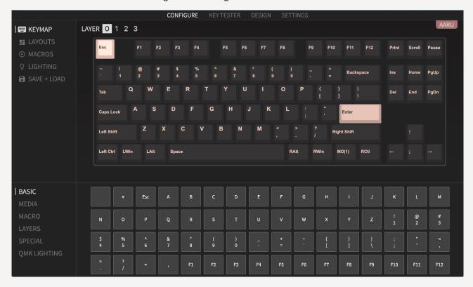
0 1 2 3 located at the top of the upper chart marks the layer, click on "1" to modify the second level key value.
