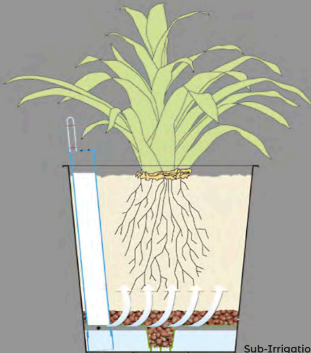
Sub-Irrigation System by ArchitecturalSupplements
