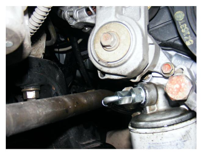
This plug is damn near impossible to remove without breaking the loctite bond by heating to over 400F.
