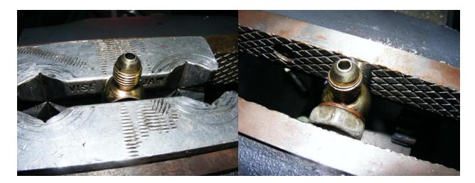
Holding the banjo fitting like above you can now tighten the line to it without damage that leads to a leak. You want to tighten the line to the fitting now because wrench access is very limited in that area once the turbo is in the car.
