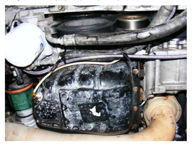
Tighten filter body, JIC ¼" union to filter body, attach filter body to hose end, tighten. Use zip ties and clamp to hold filter under radiator core support. Filter is placed in this position (under radiator area) to allow easier servicing. Filter has a special orifice size for this application, .070". Also note line zip tied to P/S hard line, this allows OEM undertray attachment point to fit.
