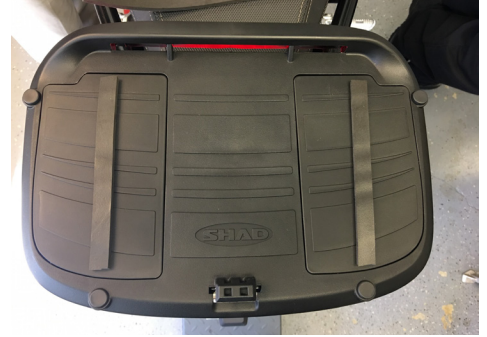
Figure 17. Foam Strips For A More Silent Ride
