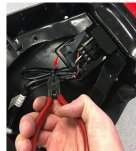
Figure 6. Cable Tie Location
