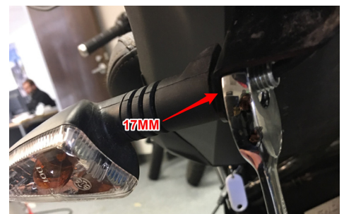
Figure 4. Turn Signals Detached
