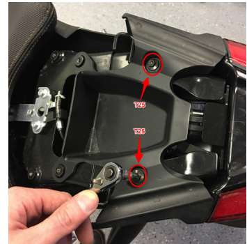
Figure 5. Seat Tray Removal
