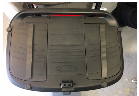
Figure 26. Foam Strips For A More Silent Ride
