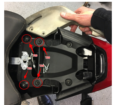
Figure 2. Grab Handle Removal
