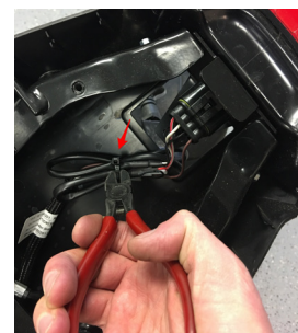
Figure 6. Cable Tie Location
