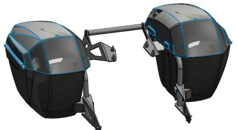
Image 3. SR/F Side Rack Assembly and Cases
