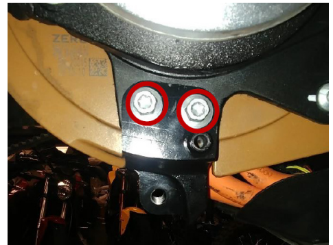
Figure 3. Centerstand Pivot Plate Right Installed
