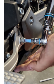
Figure 9. Brake Pedal Bolt Torquing
