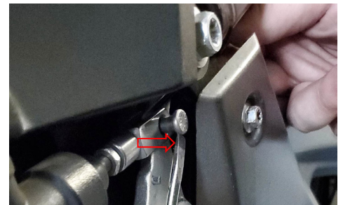
Figure 7. Remove Brake Pedal Clevis Pin
