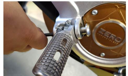
Figure 2. Removing Clevis Pin
