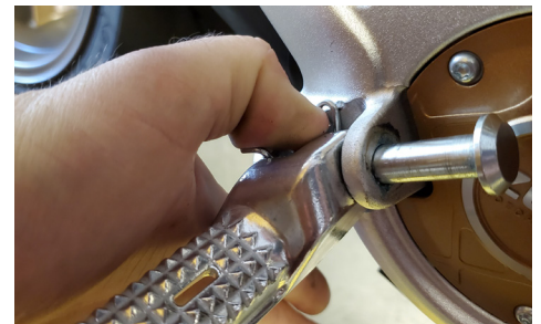
Figure 3. Attach New Footpeg with Clevis Pin
