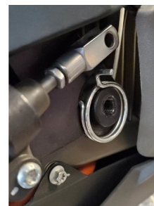
Figure 8. Brake Pedal Bolt Removed
