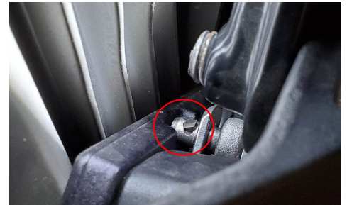
Figure 6. Compress Pin on Brake Pedal Clevis Pin
