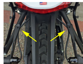
Figure 19. Signal wire secured to rear support
