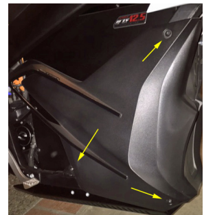
Figure 6. Remove battery fairings
