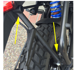
Figure 12. Right rear support attached
