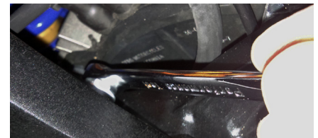
Figure 7. Right side access to footpeg bracket
