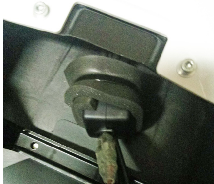
Figure 3. Rear ferrite wrapped in foam
