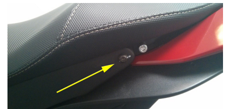
Figure 1. Seat bolt location
