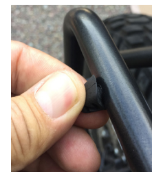
Figure 24. Bumper pressed into place
