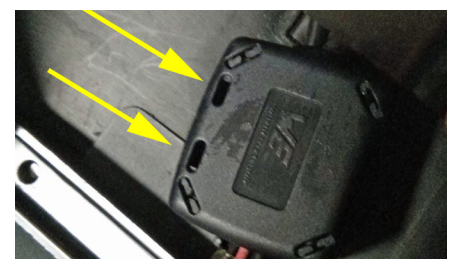
Figure 4. Holes for removal of ferrite
