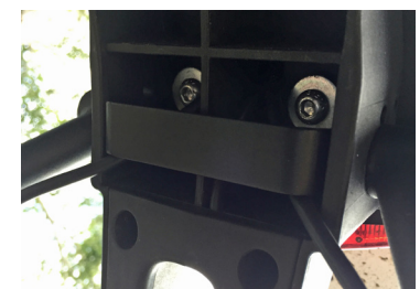
Figure 13. Crossmember placement from below
