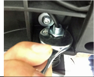
Figure 5. Remove turn signal hex nuts
