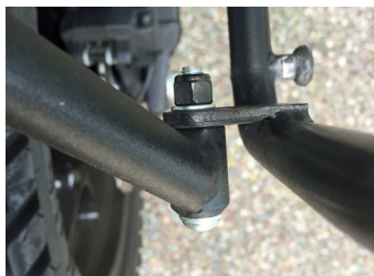
Figure 14. Lower rear supports to weldment
