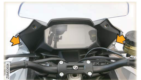
Figure 3. Remove short bolts (2x)
