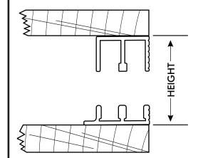
Use screws to fasten track and guide to mounting surface.
