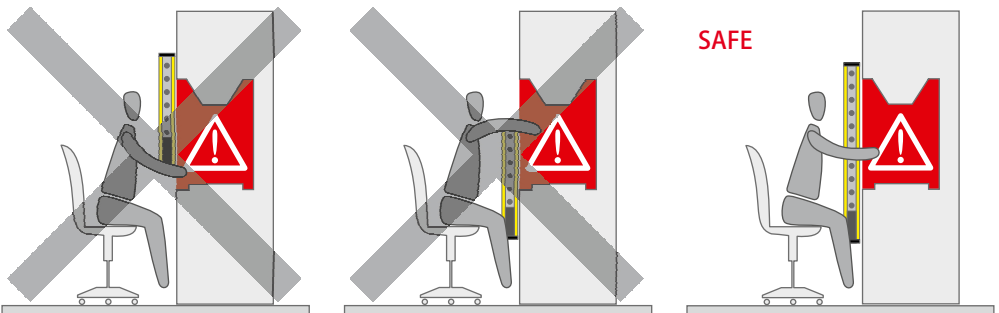
FIG. 9: POSITIONING THE LIGHT CURTAIN
