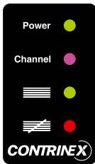
FIG. 8B: LED INDICATORS ON RECEIVER UNIT
