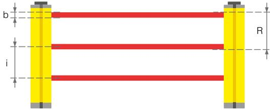
FIG. 7: RÉSOLUTION (R) OU CAPACITÉ DE DÉTECTION D'UN AOPD
