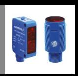
Standard C23 and M18P series are high quality ASIC sensors with an integral IO-Link interface that makes them particularly suitable for smart factory applications. Background suppression types feature a pinpoint LED and special Contrinex optics that provide excellent characteristics and long sensing ranges (up to 300 mm on white and gray, 250 mm on black). Very high accuracy and reliability make them ideal for general positionand presence-detection in almost any industry.
