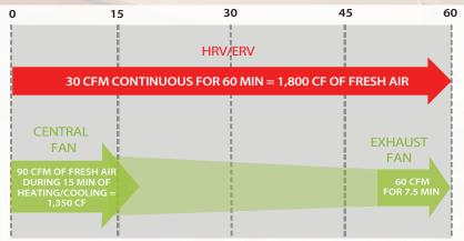
1,800 CF of fresh air required - 1,350 CF provided during heating/cooling = 450 CF still needed
