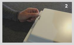
Insert S-hook at each end of the heater.
