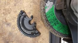
**Step #5:** Once you have the old gear removed, you will grind the mushroom head of the shaft down to the knurled diameter or less. It is very important to grind the ENTIRE TOP smooth. If not, you will crack the gear during installation. The new gear is not defective and most cases of breakage are a result from the installer not grinding down the mushroom head completely on the end of the shaft!!
