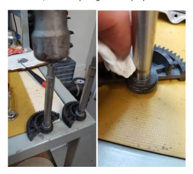
**Step #7:** Remember to put the washer on at this time so you don't forget. Insert the shaft back into the housing and hook the return spring into the slot of the half gear. Spin the gear one revolution to tension the return spring properly. Fully seat the shaft and gear into the housing allowing the gear to rest on the internal metal stop.
