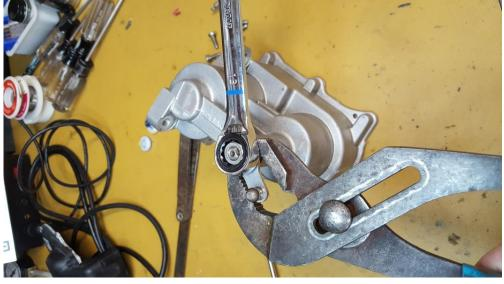
**Step #3:** Use the flat side of the channel lock pliers to lay flat across the top of the shaft and strike hard with a hammer to drive out the shaft. The idea is to not mess up the threads. If you have a large enough press, use that over a hammer please!!
