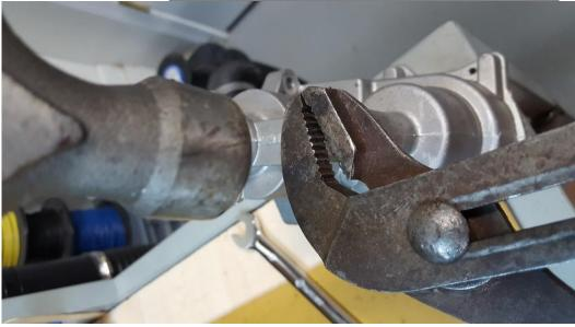
**Step #4:** Remove the shaft and take note of the washer that needs to go back on during reassembly. Use an angle grinder or Dremel style tool to carefully cut the old gear off the shaft. It was encapsulated on when originally molded. This was to prevent the shaft from backing out while in use.
