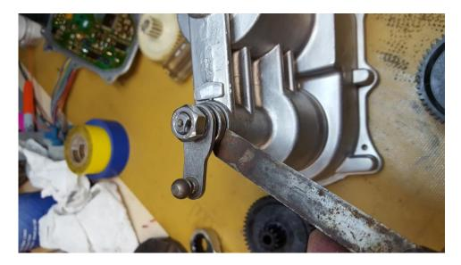
**Step #2:** Use channel lock pliers on the lever arm to keep the half gear off the metal stop. A box end wrench, 13mm, will take the locking nut off the top of the shaft. Yes, we don't care about the original gear since it is worn but this will be good practice on reassembly to not put pressure on the new gear when tightening the nut.
