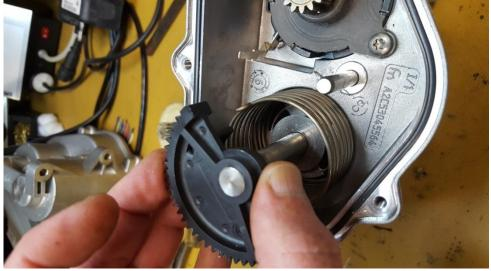
Step #8: Place the thin washer and the locking washer back on the top portion.
