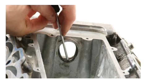
7. Carefully clean the front seal gallery. Lubricate all surfaces of the front seal liberally (item#8) with the grease provided in the kit (item# 6).
