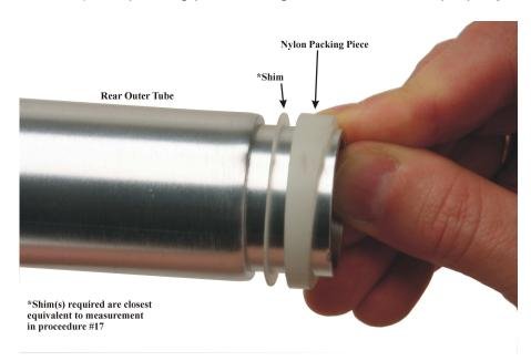
19. After re-seating the tube in the block the lock ring groove should now be exposed with no slop; push spiral lock ring forward into grove locking tube in place.
