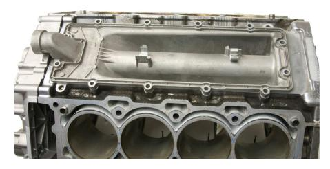
2. Remove the intake pan so the factory 1 piece coolant pipe will now be exposed.
