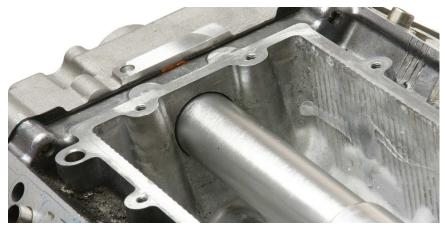
13. With a soft faced pry tool, lever the tube forward until it stops against the timing cover.
