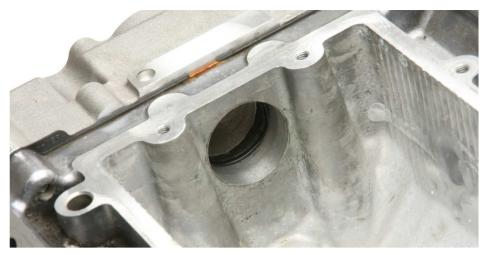
9. Perform the same lubricating and fitting operation to the rear o-ring; (item# 9); noting however there is no orientation necessary for this seal.
