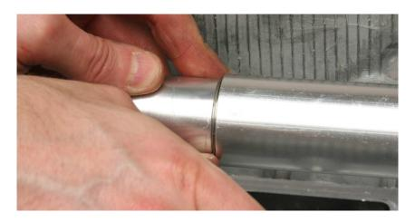
\*Only as required: If after fully seating the tube into the block the snap ring groove is beyond the end of the rear tube half, installation of shims will be required. Casting variations during block manufacturing may make this simple procedure necessary.
