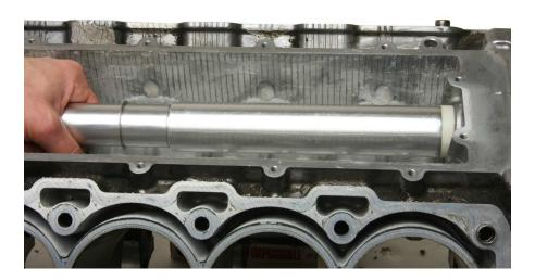
15. Grabbing both sections of the tube firmly, hold the front half in place and slide the rear section back into the block until it clicks home.
