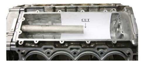
\*Important note: Care must be taken at all times to keep debris and cuttings out of the engine.
