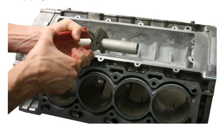
5. Remove the remaining front seal material with a pick and wire brush taking care not to damage the seal housing.
