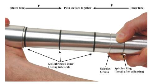
Then install the Spirolox (item# 7) around the smaller inner tube and position it by sliding it up against the end of the larger outer tube.
