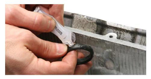
8. Fully fit front seal (item#8) into housing taking care to make sure the \*flat profile of the seal faces the timing cover (forward). (\*this is critical to a proper installation).
