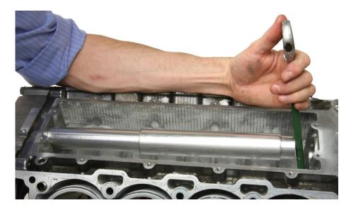
14. Fit rear white nylon angled packing piece (item #3) onto the back end of the water tube with the flat side against the water pipe shoulder and with wide angle facing upward. Lubricate the end of the larger outside tube with grease provided.
