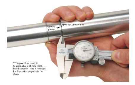
18. Slide rear tube section forward again, remove the nylon packing piece and fit the appropriate shim stack (item #4) (equaling the previous measurement) refit packing piece taking care to orientate it properly.
