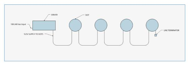
To help with larger system there is a splitter accessory. This enables a Y-split in the wiring. All lines must be terminated for the system for function correctly. An additional terminator is included with each splitter. Note high numbers of splits in a system can increased to complexity of fault troubleshooting.
