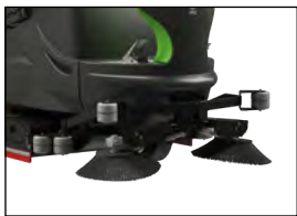
PRE-SWEEP SYSTEM ON CYLINDRICAL MODEL
