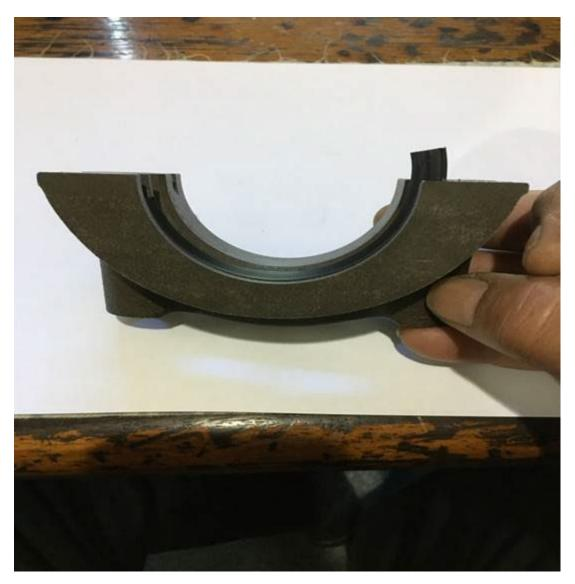
Once you have applied the sealer on the back of the seal place each half in the block and cap with the seal offset about 10 mm
