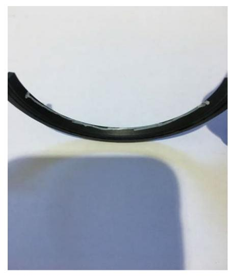
Apply some rubber grease or Vaseline in the area marked in white marker do not go to the edge of the seal about 10mm from each end is plenty.
