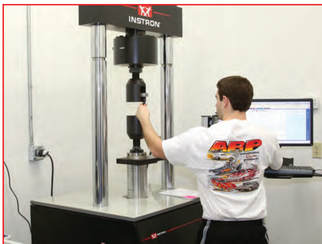
Two computer-controlled Instron tensile machines are used to determine the ultimate tensile strength of studs and bolts.
