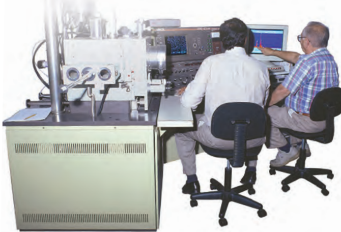
ARP engineers use "Scanning Electron Microscopic" inspection capable of detecting all elements in the periodic table with atomic numbers greater than 5 – permitting the acquisition of high resolution imaging.
