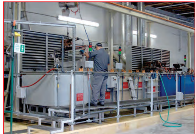
The finishing touch for most chrome moly fasteners is the black oxidizing operation. Fasteners go through a series of "baths."
