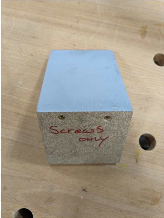
Screws only, no glue. Stronger join than MDF. Painted over the butt joint, no visible join
