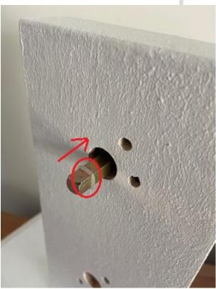
4. Insert O-ring over spindle, and using a small screw driver push this O-ring inside the hole so it falls within the grooves in the spindle.
