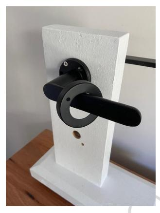
11. Slip rose cover plate over both internal and external handles ensuring the privacy pin hole is sitting horizontally on the latch side, and push on until sitting flush against the door.
