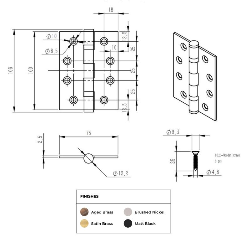
Fixings: Supplied with 16 x Timber Fixing Screws in matching finish.
