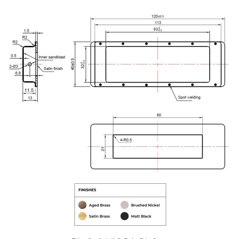
**Fixings**: Supplied with 2 x Timber Fixing Screws.
