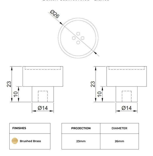
Fixings: All single-fix cabinet handles are supplied with 1 x 25mm M4 fixing screw.
