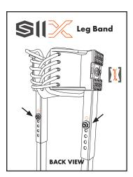
**The S2X Rocking Leg Bands** have 2-3/4" of height adjustment. Simply remove the bolts and align with additional holes in side poles. There are two holes on the inner side poles (holes that cannot be seen until bolts are removed - (1)). Use these holes to achieve maximum height. Secure bolts before use.
