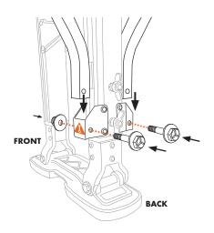
First, match Left and Right Leg Bands to Left and Right Stilt bodies. Insert Lower Strut Tubes into the two Outside Brackets on the main stilt body. Insert bolts with washers and attach nuts. Leave loose until side pole holders (item A on next page) are positioned into side pole bracket (item B on next page). Fasten poles securely using 11 mm wrenches before use.
