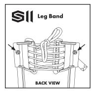
**The S2 Leg Band** can be raised and lowered if needed. Simply remove the bolts and slide the leg bands to align with additional holes in the side pole. These holes cannot be seen until bolts are removed and the Leg Band is repositioned. Secure bolts before use.
