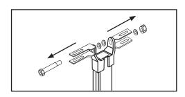
Then, thread the straps through the top portion of the footplate, and secure in place with panhead screws.
