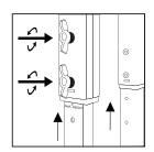
**Caution:** Do not pull the Inner Extension Tube past the "Max. Height" engraving, or force the Inner Extension Tube out of the Main Leg Strut. A plastic sleeve and tab is present to prevent this from happening, but excessive force will damage the plastic sleeve.
