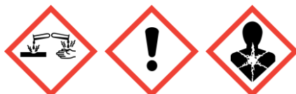
Corrosion Exclamation mark Health hazard
