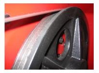
13- Turn the hand-wheel to right (tensioning position) to exert sufficient tension on the saw blade.
