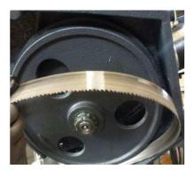
**6.** Place the sawblade between the bearings.
