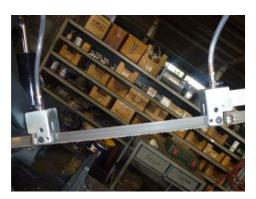
**9.** Tighten the sawblade with tensioning shaft.
