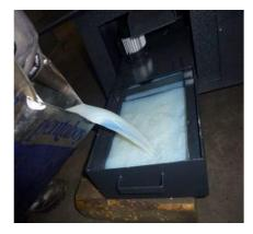
**4.** Placing the coolant tank.
