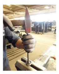
5) Hammer pin into the bearings
