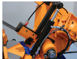
Control your downfeed to suit the material you are cutting
