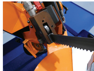
Carbide Guides - gives you more accurate cuts and longer blade life
