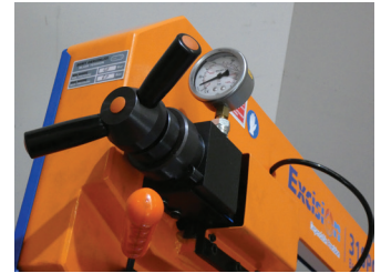
Blade tension gauge - having the correct tension saves broken blade and crooked cuts
