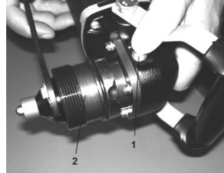
1 = Release button. 2 = Drive shaft.
