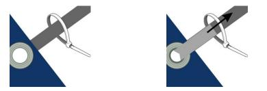
**STEP 2:** Pull cable tie to tension, the straps should not be able to slide- you can trim the cable tie but allow for 5-10 mm of length to enable reuse.
