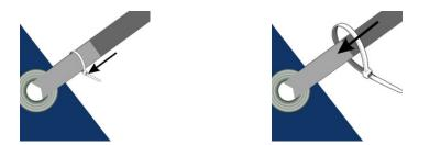
**STEP 3:** Thread the side strap nearest the foot end of the table through the T strap as shown and tighten. Next, feed the strap and end of the bed through the single loop and tighten. Use the cable ties as shown above for all fixing.
