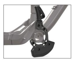
4. WASHERS CAN BE USED TO FINE TUNE YOUR SET UP TO GET THE CORRECT CHAINLINE. WE HAVE SUPPLIED MORE WASHERS THAN YOU REQUIRE TO ENSURE YOU CAN TAILOR YOUR SET UP. THE CHAIN SHOULD SIT IN THE CENTRE OF THE GUIDE.
