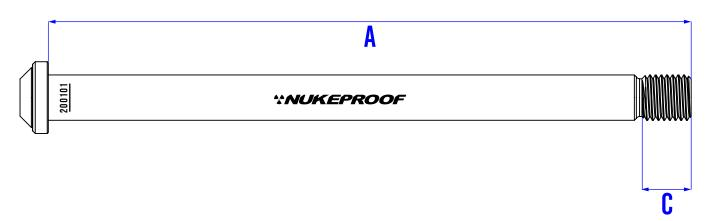
TO DETERIME REAR THREAD PITCH (B), PRINT PAGE AT 1:1 WITH NO SCALING AND SET YOUR OLD AXLE ON TOP OF THE PRINTED THREADS TO SEE WHICH THREAD PITCH YOU REQUIRE. IT CAN BE DIFFFICULT TO DETERMINE THE THREAD PITCH SO CLOSE ONE EYE AND LOOK DIRECTLY DOWN THE THE AXLE. CHECK THE WHOLE THREAD TO ENSURE THE THREAD MATCHES THE PAGE.
