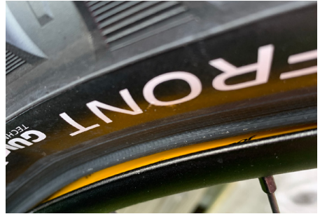
14. Finish fitting tyre. Make sure the bead is pushed to the centre of the rim as this will make it much easier.
