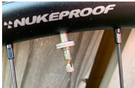
4. When the tube is deflated, remove the nut holding the valve in place.
