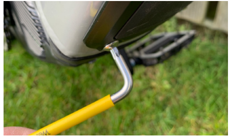
16. Tighten the lower left bolt using a 4mm hex key
