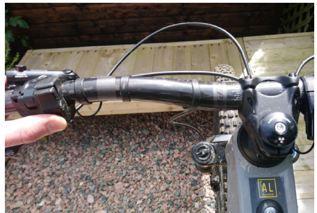
Walk - Press and hold bottom shifter button to engage walk mode. Motor will provide assistance to make pushing the bike easier
