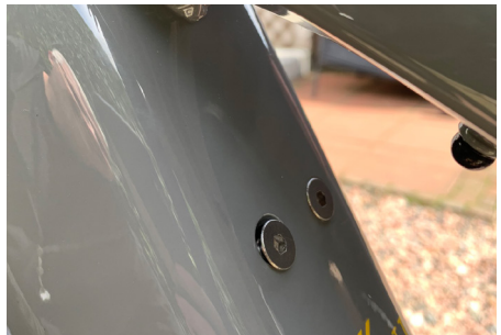
16. Move cables into correct position and then tighten battery mount bolts – be careful not to pinch any cables as you do this
