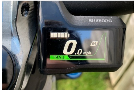
Trail - Perfect for general MTB use and safest for steep descents. A couple of turns of the cranks are required for the motor to provide assistance
