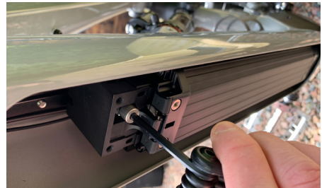
4. Carefully turn the battery release hex clockwise to release the battery. It will slide forward onto a secondary catch which you will need to push down to fully release and remove the battery.
