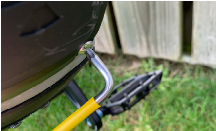
17. Tighten the lower right bolt using your 4mm hex key
