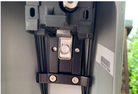
15. Put the battery mount back into the frame and loosely insert bolts
