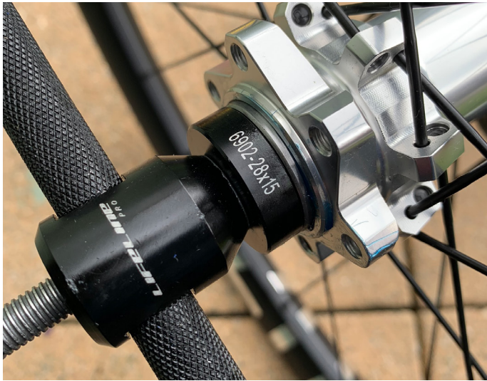
11. Carefully put your bearing press through the bearing & hub. Use the correct size of bearing drift and press in the bearing
