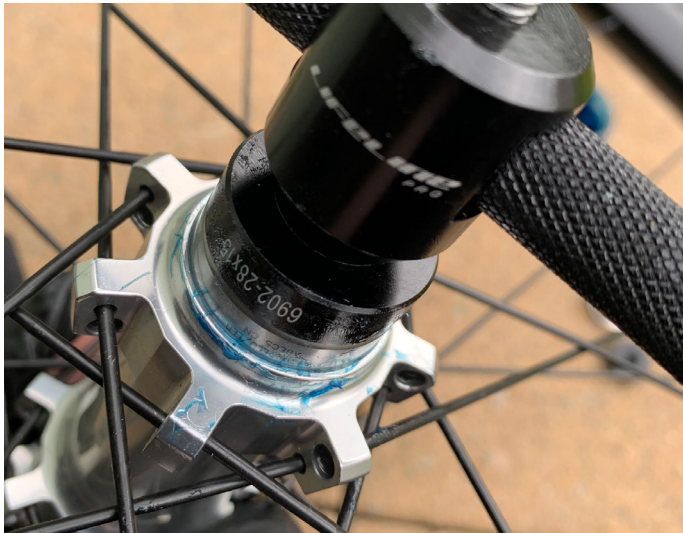
13. Carefully set the other bearing into position on the hub shell then put your bearing press through the bearing & hub. Use the correct size of bearing drift and start to press in the bearing. Note: If you are using the Nukeproof Enduro bearings, the blue seal faces outwards
