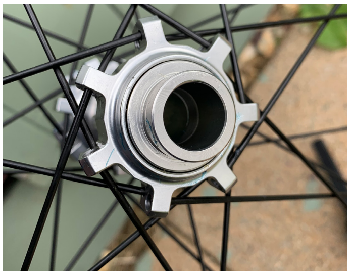
16. Refit your driveside end cap by pushing it into place
