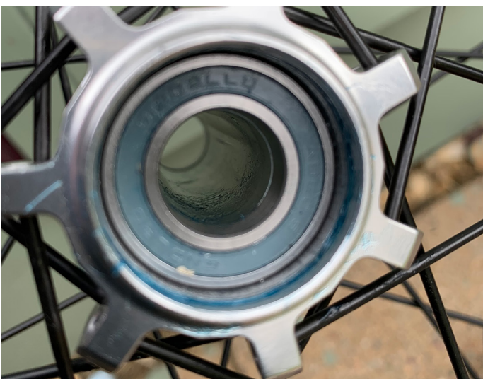
15. Continue to finish pressing the bearing so it has been fully seated correctly
