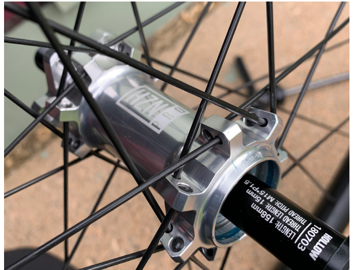
14. As the sub axle needs lined up, it is important to STOP pressing in the bearing when you start to feel resistance. At this stage get your fork thru axle and put it through the hub to line up the sub axle
