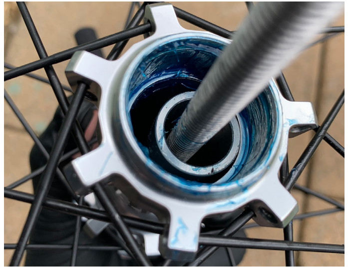
12. Put the sub axle back into the hub
