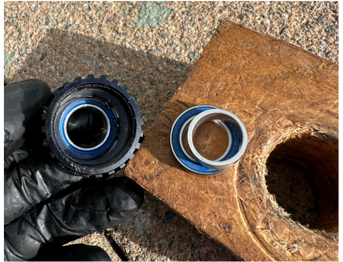
18. The bearing & spacer should now be removed from the hub
