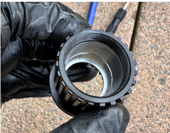
21. The freehub should now have all bearings removed and inspected to ensure there is no damage and it is visibly in good condition.
