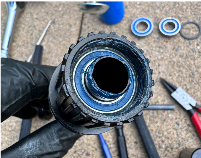
31. Put the axle through the freehub to get the bearing spacer lined up correctly
