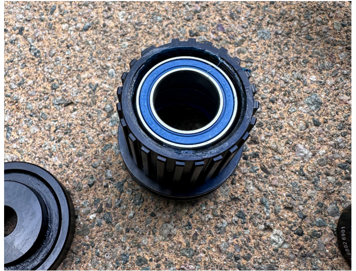
24. Get your bearing, apply grease then set it in place
