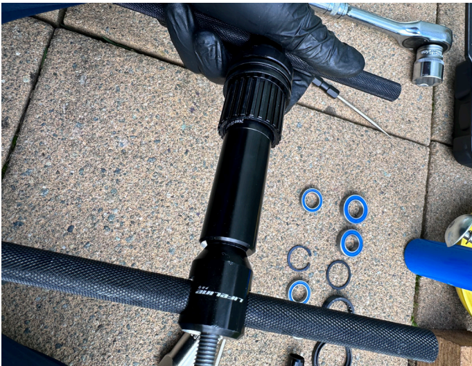
25. Press the bearing into the freehub with your bearing press
