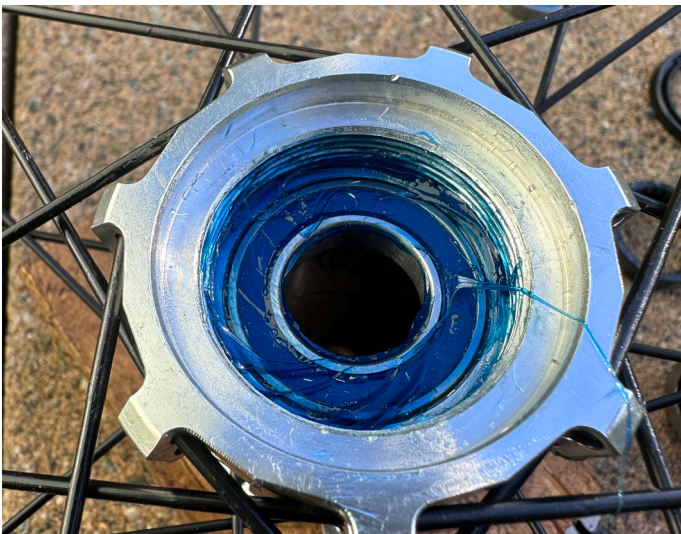
37. Apply grease to the outside of the bearing
