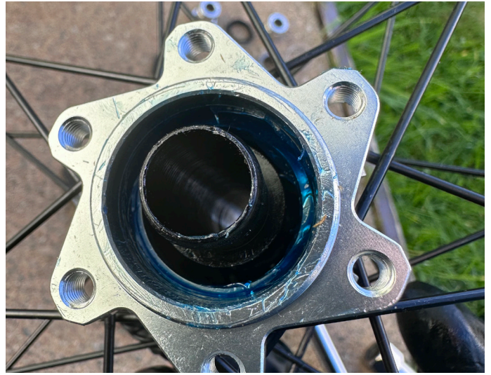
42. Insert the axle into the hub, ensuring the longer part goes to the drive side
