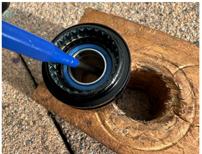
16. Get your freehub and using the bearing punch, push the inner spacer so it exposes the rear of the outer bearing
