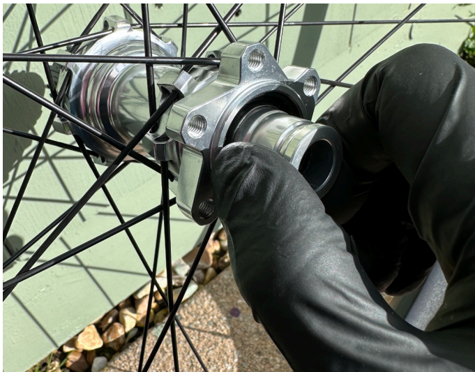
1. Pull off non-drive side end cap
