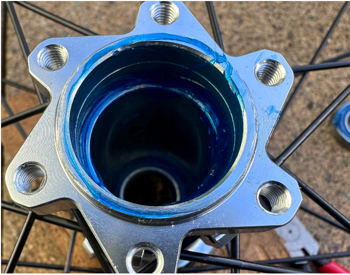
41. Apply grease to non-drive side bearing seat
