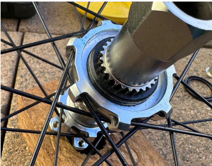
39. Install the inner ratchet nut and tighten
