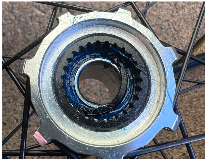
40. Ensure that washer is not visible, if it is like the photo, loosen the nut to reposition the washer then tighten it again
