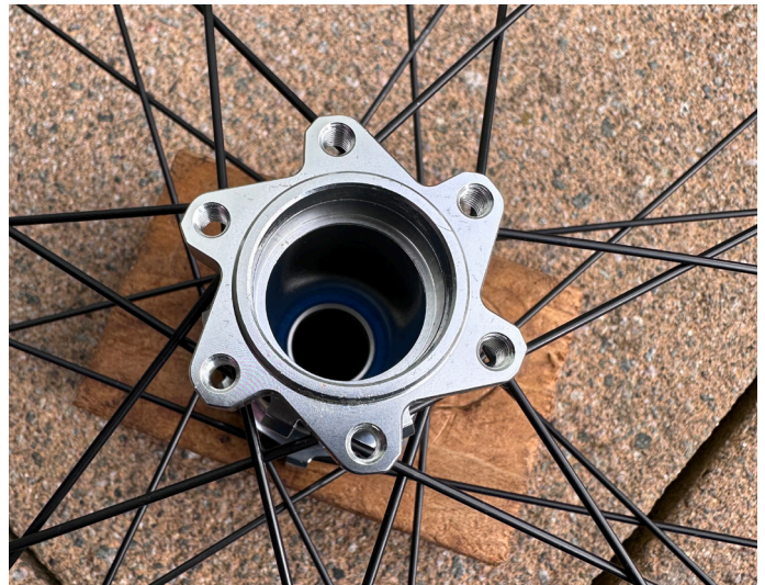
14. Turn over the hub so the drive side is now on the hub support
