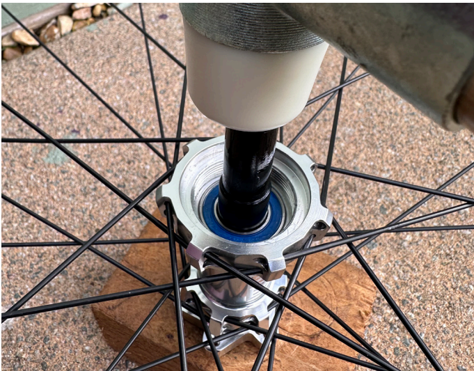
13. Hit the end of the axle with a hammer to remove the non-drive side bearing
