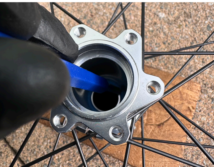
15. Using a bearing punch, gently tap the bearing to remove
