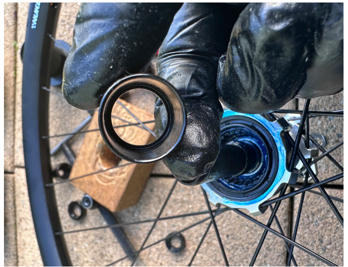
50. Refit bushing to axle – Note this can only be fitted one way and should cover the thicker part of the axle
