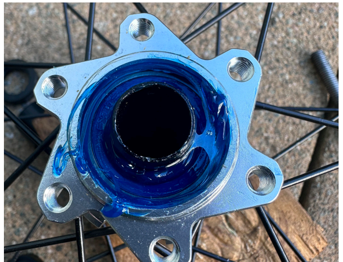
44. Apply grease to the outside of the non-drive side bearing
