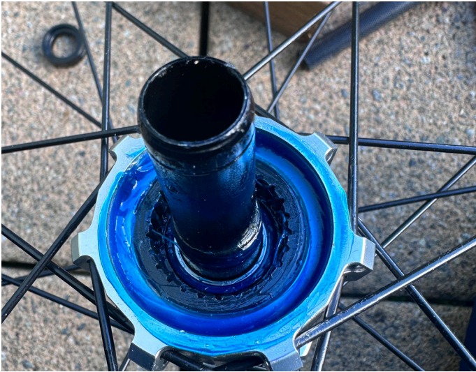
47. Apply grease to the drive side seal seat
