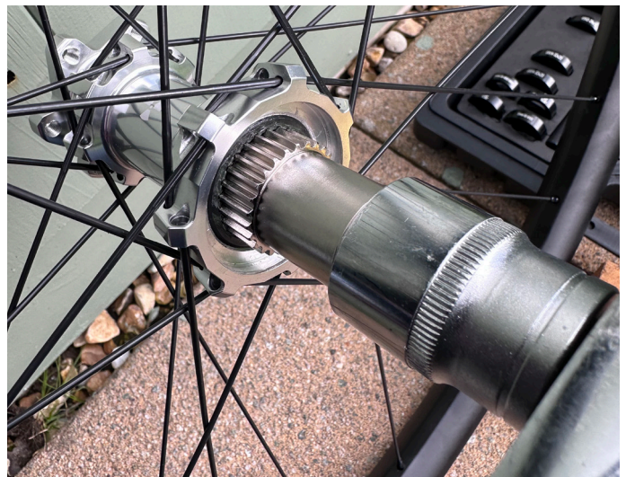
10. Using the inner ratchet tool, remove the inner ratchet. Depending on your specific tool you will either need to place the tool upright in a vice and place the wheel on top then turn the entire wheel OR use a socket to loosen and remove if no vice is available
