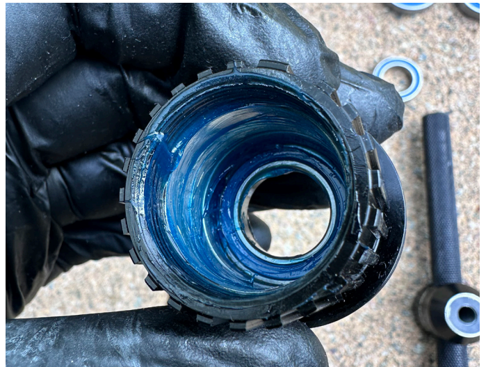
26. Apply more grease inside the freehub
