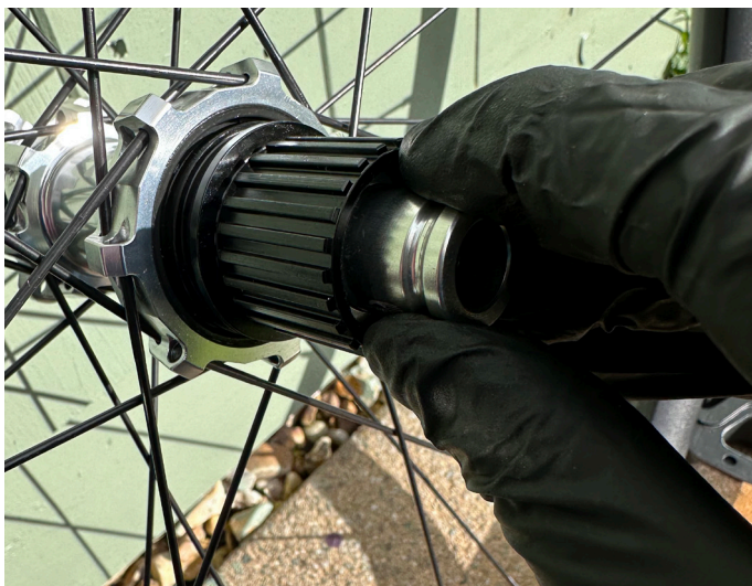
3. Pull off drive side end cap
