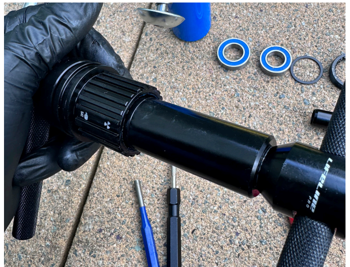
32. Finish pressing in the outer bearing
