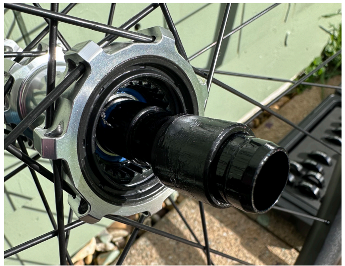
8. Take the bushing off the axle
