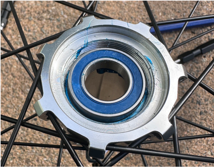
35. Get the drive side bearing and set it into place on the hub shell
