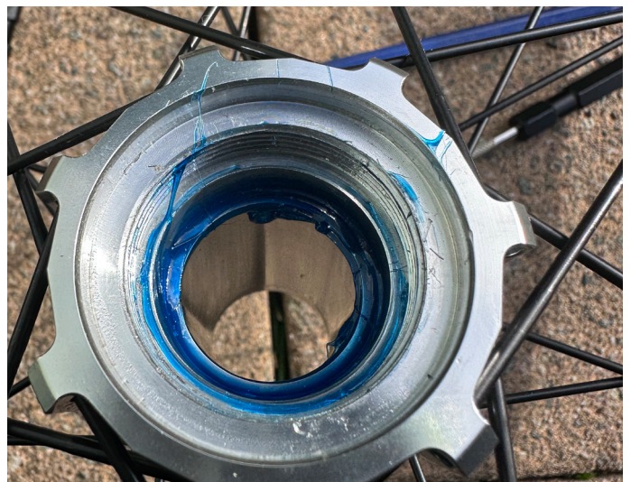
34. Grease the bearing seat on the drive side of the hub shell
