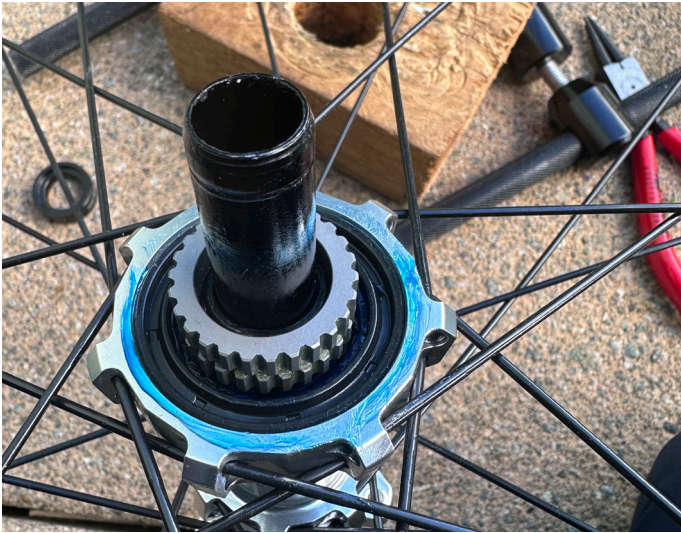
53. Refit outer star ratchet – teeth on the star ratchets should now be biting together
