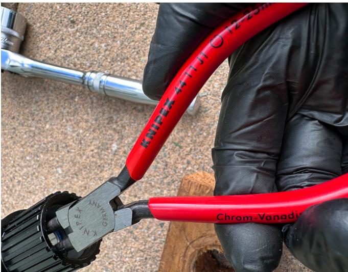
19. Using your circlip pliers, remove the circlip from the freehub
