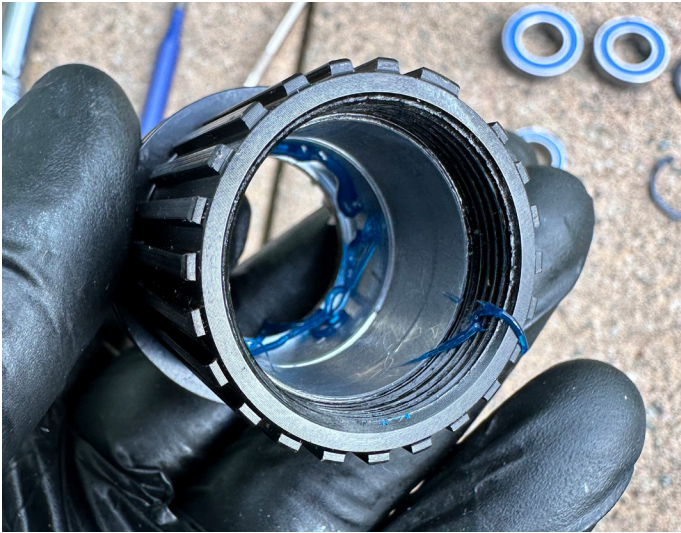
23. Get your freehub and apply grease to the inside where the bearing will be pressed to
