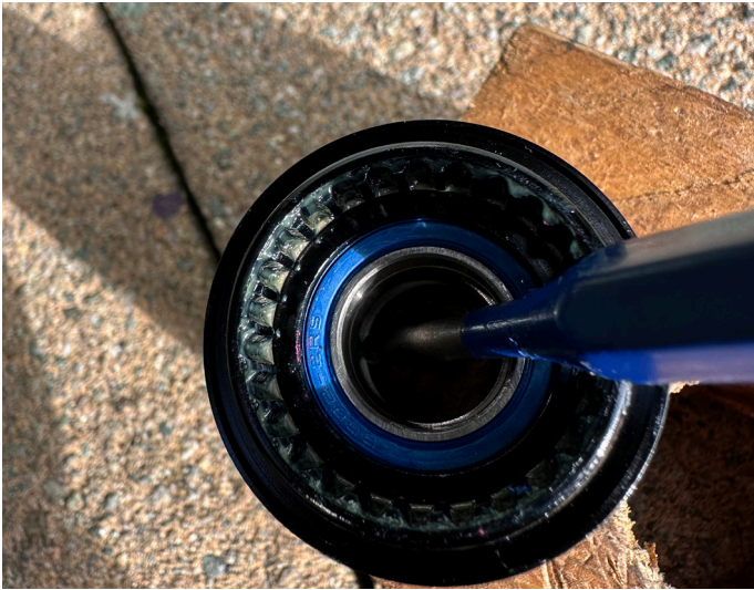
17. Using the bearing punch, remove the front bearing
