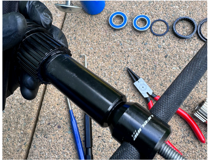
30. Start to press in the outer bearing, when it is nearly in STOP
