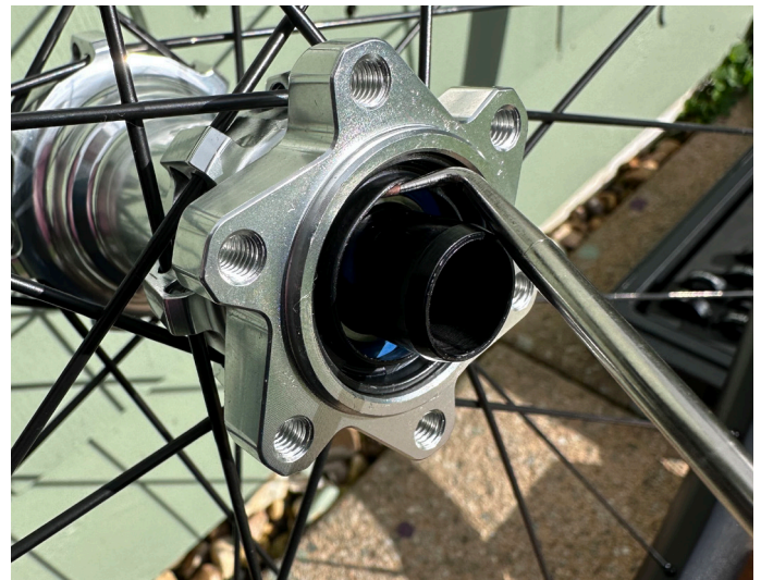
2. Remove non-drive side seal using a pick or flat-head screwdriver
