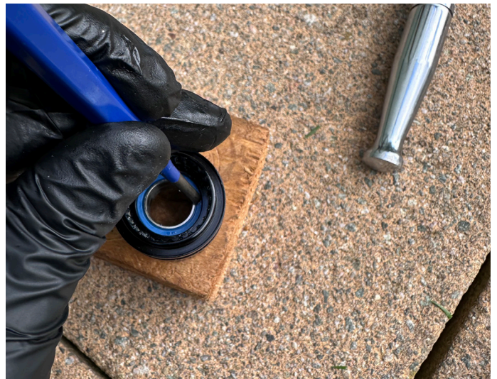
20. Using the bearing punch, carefully remove the remaining bearings in the freehub following the steps above
