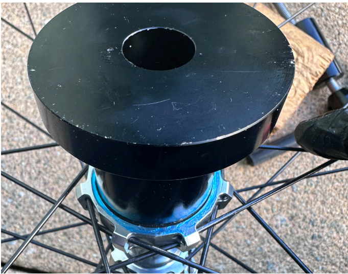
49. Push seal into hub shell using a seal press tool
