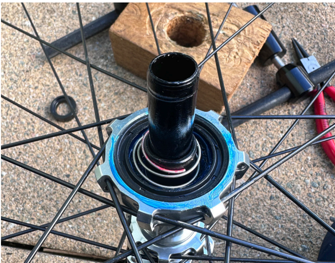
51. Refit spring – note orientation
