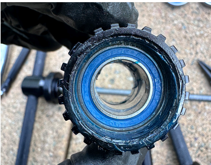
33. Your freehub rebuild is complete. If the spacer has managed to move out of place like in the photo, you should be able to push it into place with your finger
