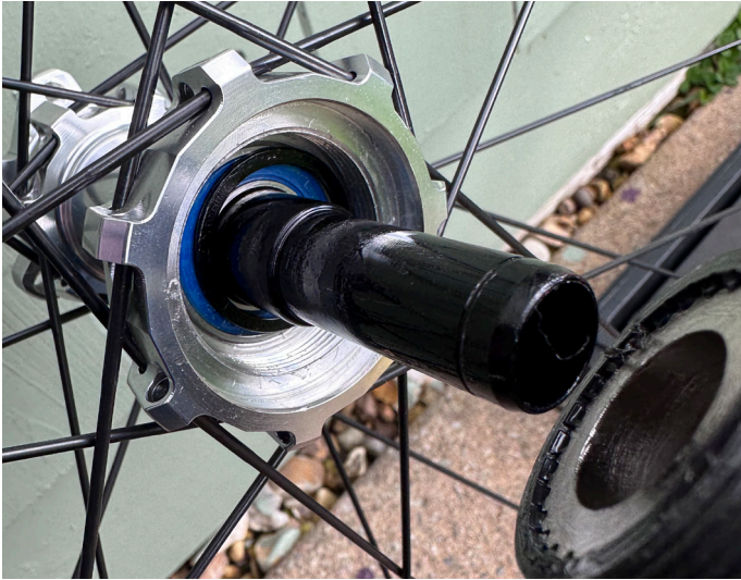
11. Remove the washer which sits between the inner ratchet & bearing
