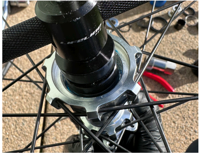
36. Press the bearing into place
