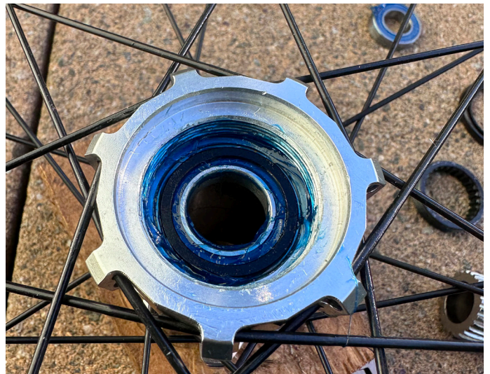
38. Get the inner ratchet washer and set it into place
