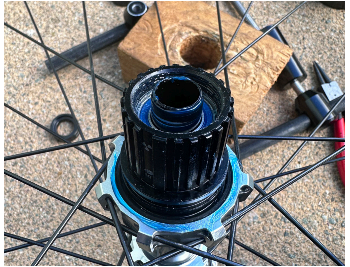
54. Refit freehub and apply grease around the outside of bearing
