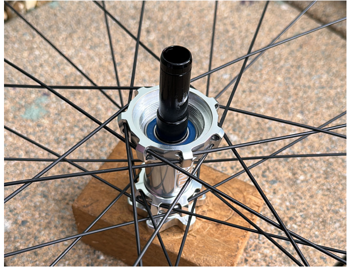
12. Place the hub non-drive side down on your hub support
