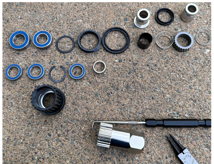
22. Your hub is now fully stripped.
