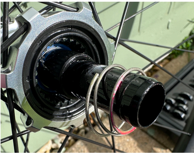
7. Remove inner spring
