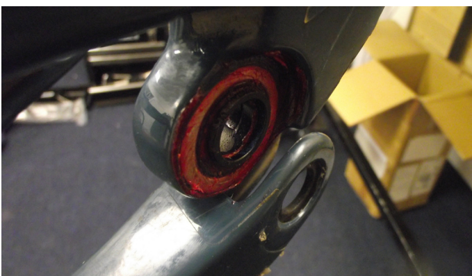
3. The Chainstay and Seatstay can now be separated, revealing the 4 Horst Link Washers (14)
