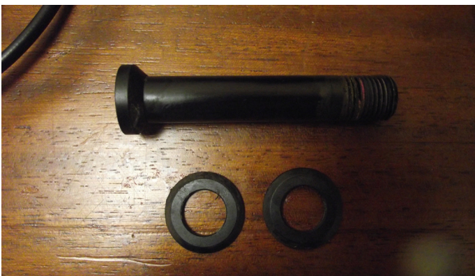
5. Removed Main Pivot Washers (11), Main Pivot Axle (21) and Collect Washer (22)
