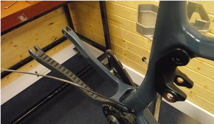
1. 29" Chainstay can now be removed
