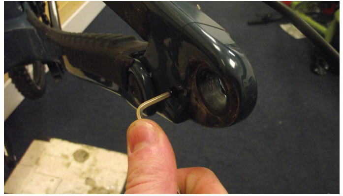
6. Remove UDH Stop Bolt with 3mm Allen Key
