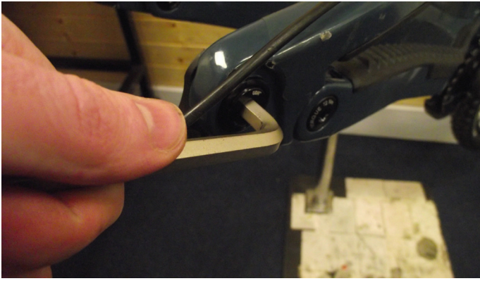
5. Remove UDH to SRAM instructions with 8mm Allen Key, note reverse thread
