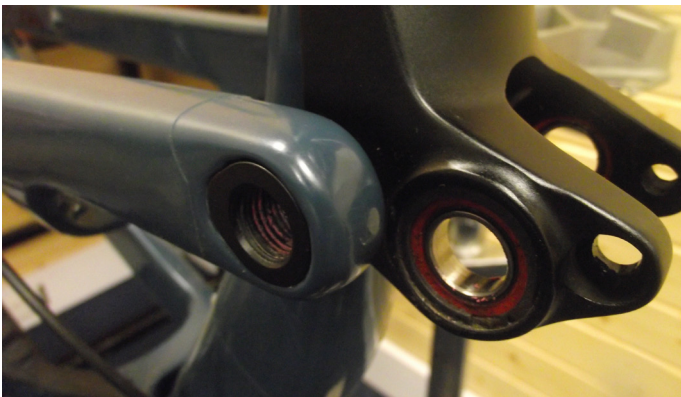
3. The Seatstay can now be removed, careful not to drop Seatstay Clevis Washers (7) and Nuts (6)
