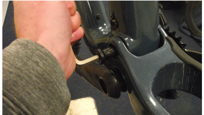
2. Remove Main Pivot Axle (21) with 8mm Allen Key
