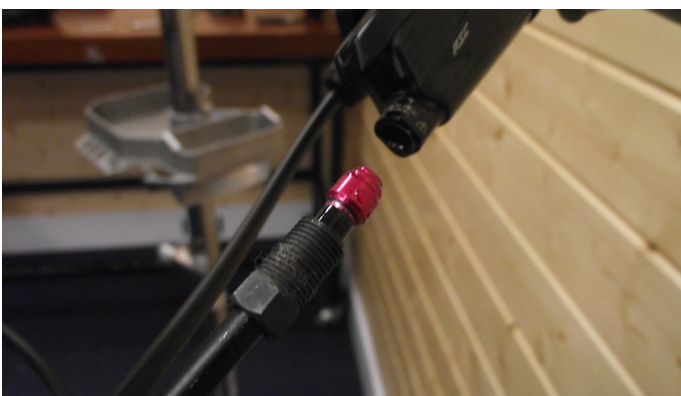
3. Remove hose from brake
