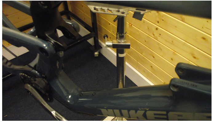
4. The Swing Link is now accessible
