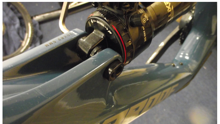
2. Remove Shock Nut Bolt (28) from frame
