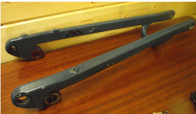
5. 29" Seat Stay Removed from bike
