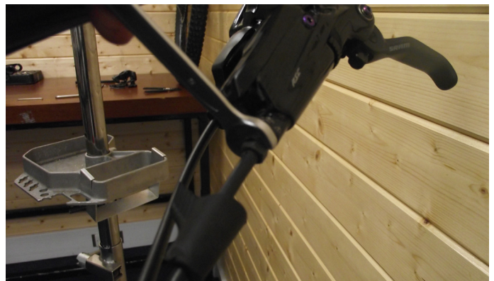
2. Partially loosen hose nut and pull hose to unseat
