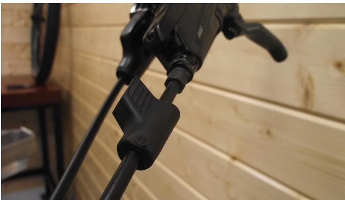
1. Remove nut cover from brake
