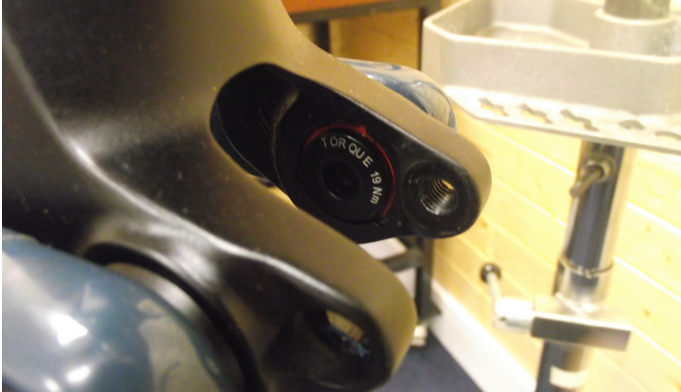
1. Seat Stay Clevis Bolts (10) can now be removed
