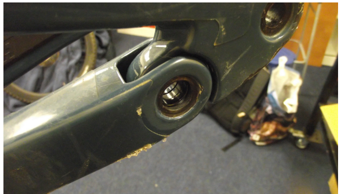
2. Horst Link Pivot and Axle (13) removed
