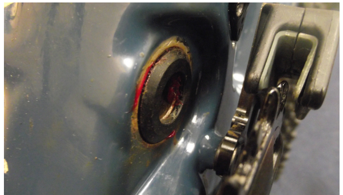
4. Remove Main Pivot Washer (11) from drive side
