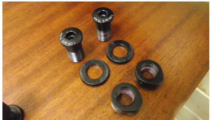
4. Set aside Seatstay Clevis Bolts (10), Washers (7) and Nuts (6)
