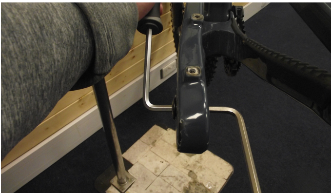
1. Using two 6mm Allen Keys undo the Horst Link Pivot and Axle (13). Note inside Allen Key stays static and outer is used for loosening
