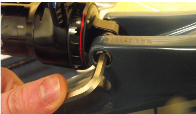
1. Undo upper shock bolt with 5mm Allen Key
