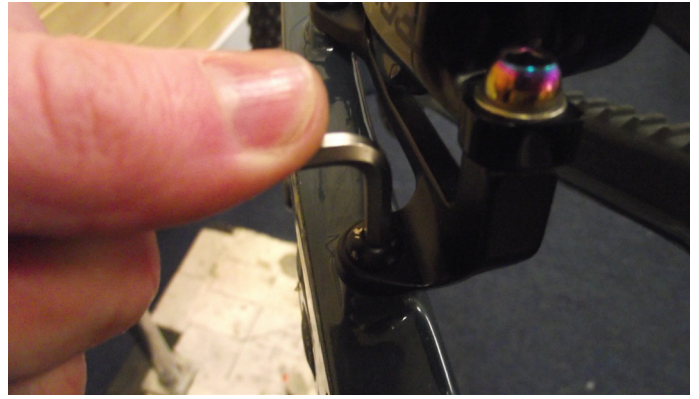
6. Undo Brake Mount Bolts with 4mm Allen Key
