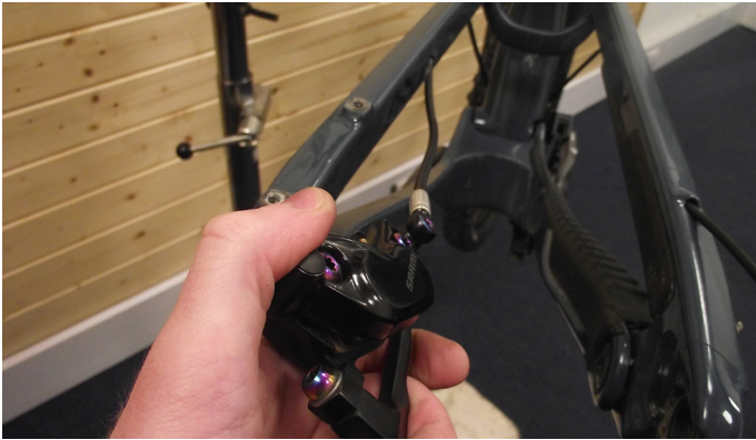
7. Pull brake hose through frame
