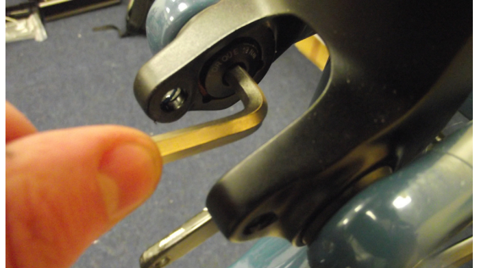
2. Using a 6mm Allen Key remove bolts from each side of the Swing Link (27)
