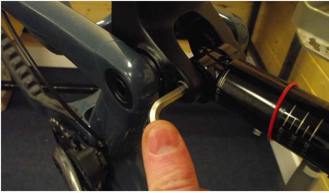
3. Remove lower shock bolt with 5mm Allen Key
