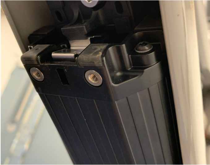
5. Push secondary clip down to fully remove battery
