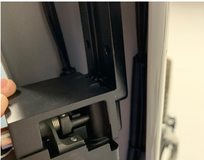
25. Remove mount inside downtube - your cables should now be loose inside the downtube
