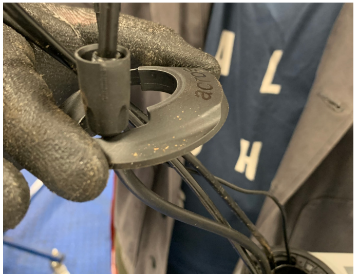
22. It is very important cables are refitted in the same position they are currently fitted. Note down their position / order and then remove top headset cover
