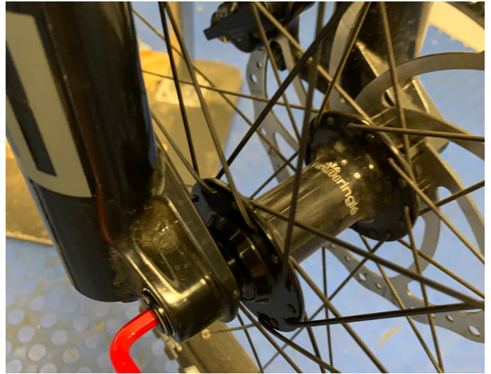
66. Refit front wheel and torque axle as per manufacturers torque setting
