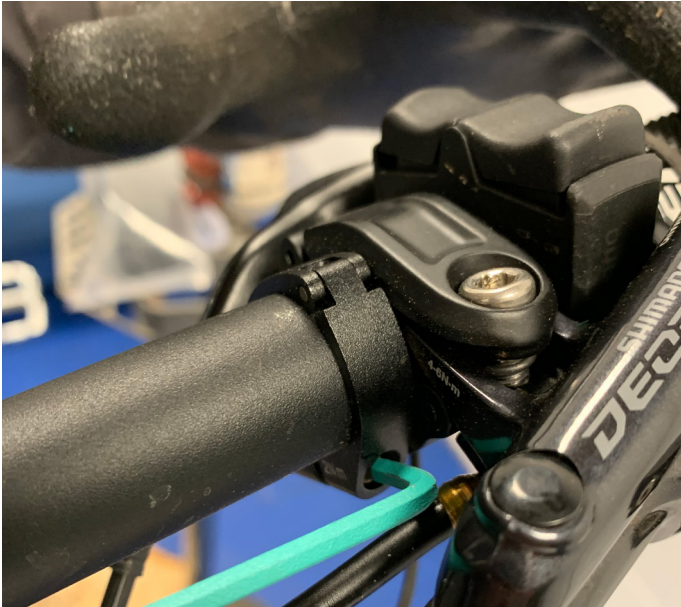
11. Disconnect dropper cable / hose following manufacturers instructions
