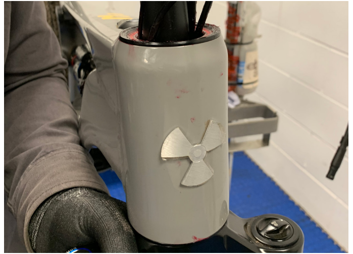
54. Insert fork into headtube ensuring cables are positioned on either side of the steerer tube
