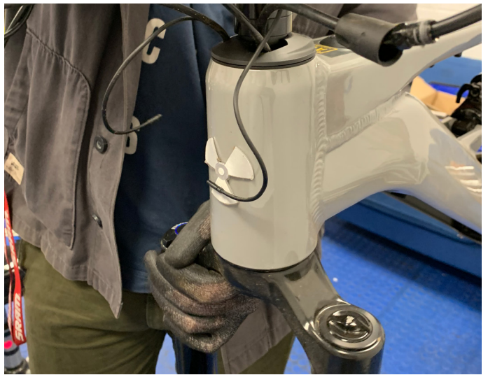
20. Hold fork by the crown and remove stem / handlebars / spacers - set somewhere safe
