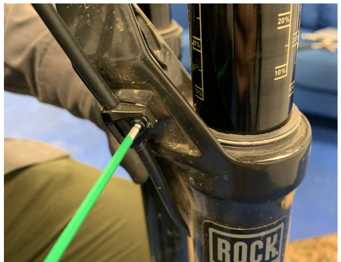
16. Remove brake hose from fork hose guide
