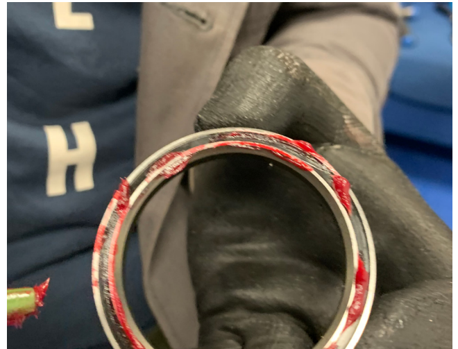
50. Insert bottom bearing (ensure chamfered edge is inside cup)
