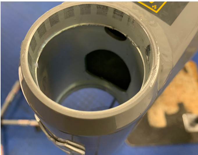
33. Clean any old grease / dirt from headtube and fork.
