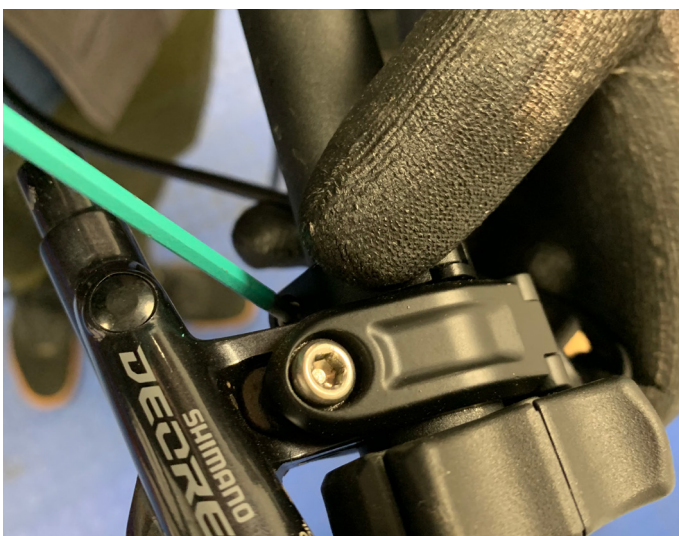
63. Reconnect dropper cable / hose - fit new cable if needed
