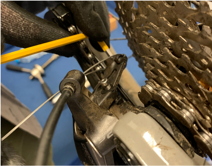
71. Tighten gear cable at rear mech and check and adjust indexing as per manufacturer's instructions
