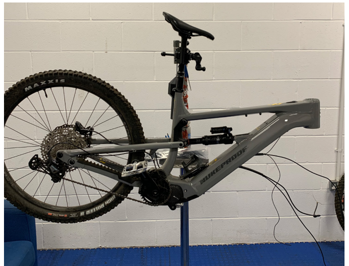
34. The old headset has now been removed from the frame and you are ready to now start reassembling
