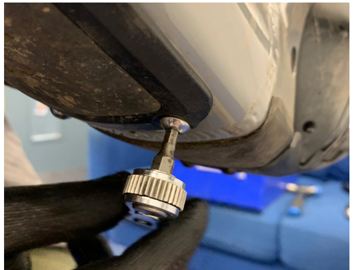
70. Tighten bottom battery door bolts
