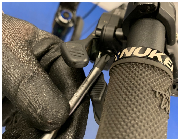
62. Refit cable cover cap on shifter
