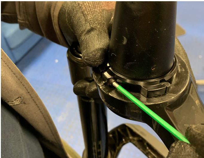
37. Ensure crown race is centered and tighten bolt to secure
