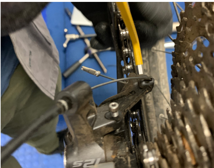
13. Undo gear cable at rear mech
