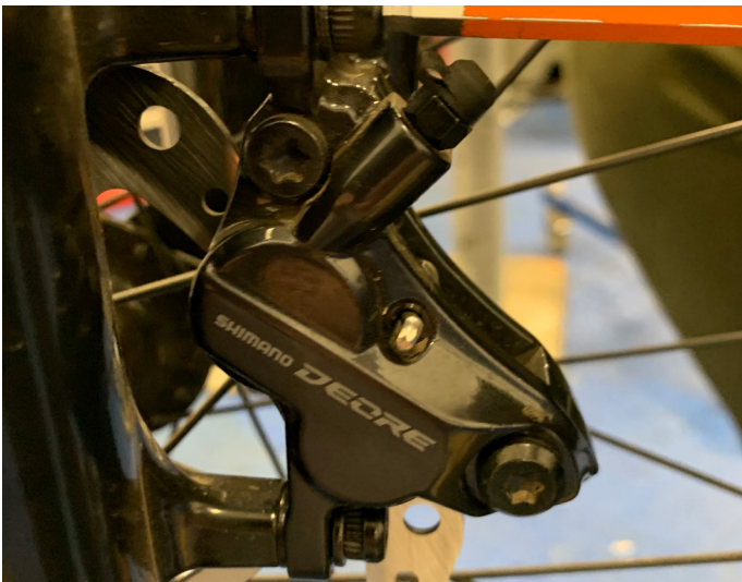
67. Align calliper and tighten to manufacturers torque settings
