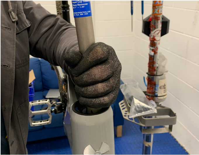
29. Tap tool with hammer to remove cup
