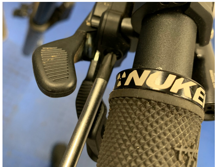
14. Remove cable cover cap on gear shifter
