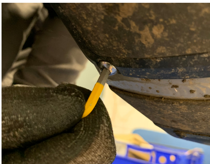
3. Loosen battery door bottom bolts 2 full turns
