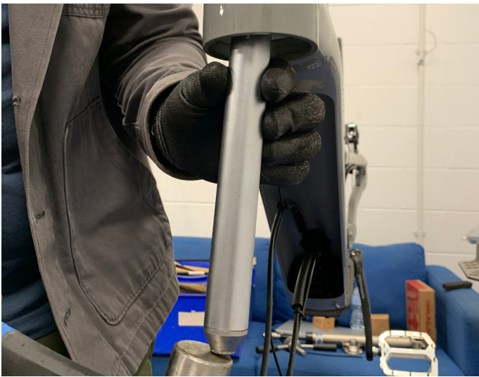
31. Tap tool with hammer to remove cup
