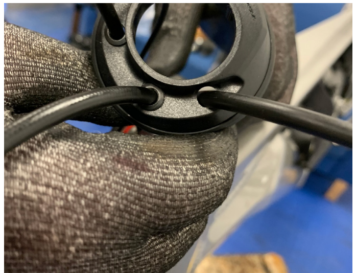
52. Feed cables through top headset cover. Use the same positions which were noted down in step 22
