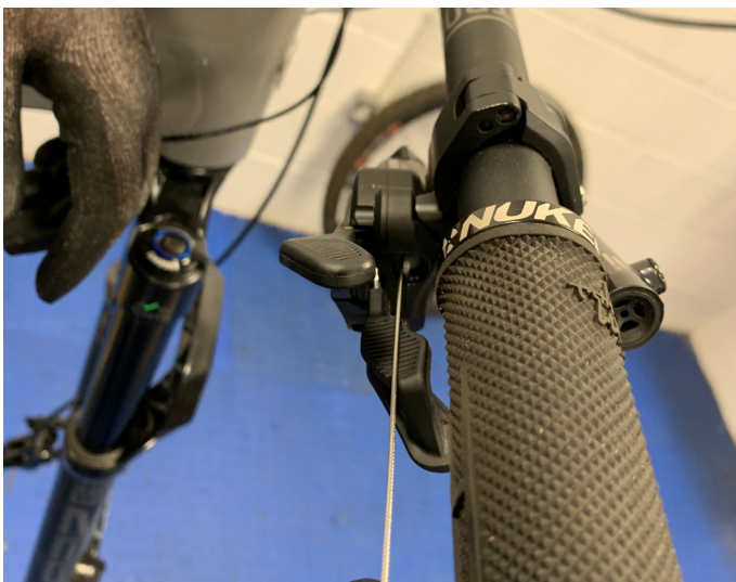
61. Insert new gear cable via shifter (leave loose at mech)
