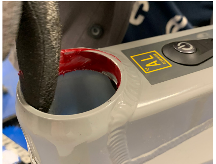
38. Apply grease to inside of the top of the headtube
