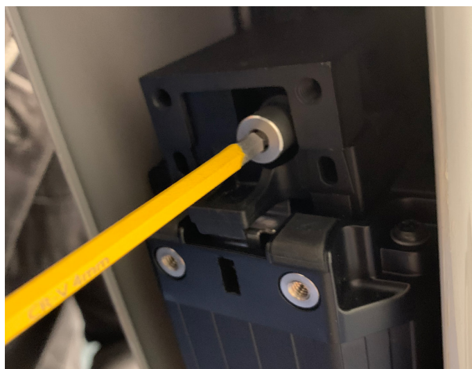
4. Remove battery by carefully turning release clockwise with a hex key, it will drop forwards onto a secondary clip
