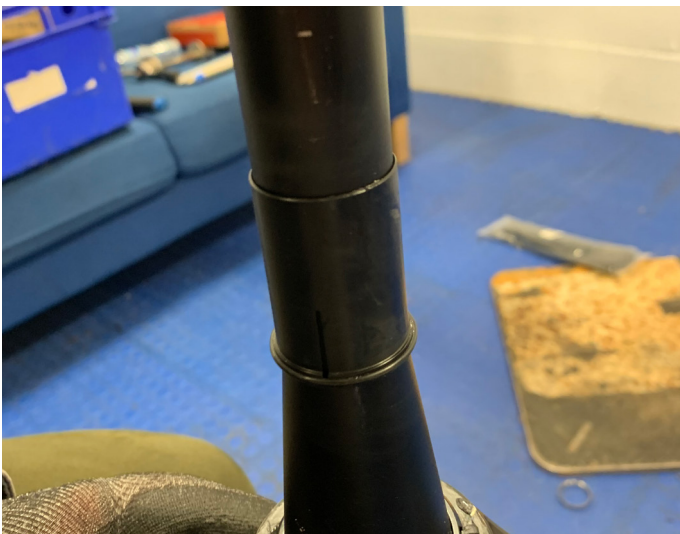
51. Fit steerer protector on steerer tube if not already fitted
