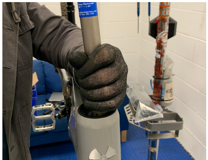
28. Insert headset removal tool for bottom cup
