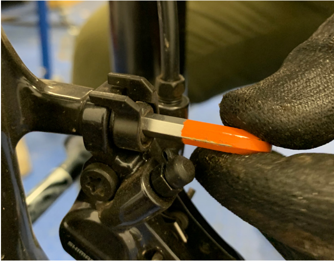
17. Remove front brake calliper
