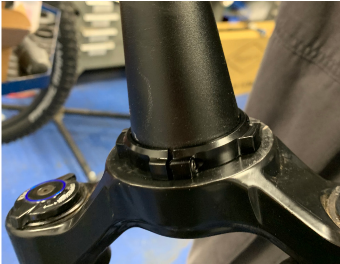
35. Add Loctite 680 around inside of crown race then then place crown race on fork - bolt hole goes to front.
