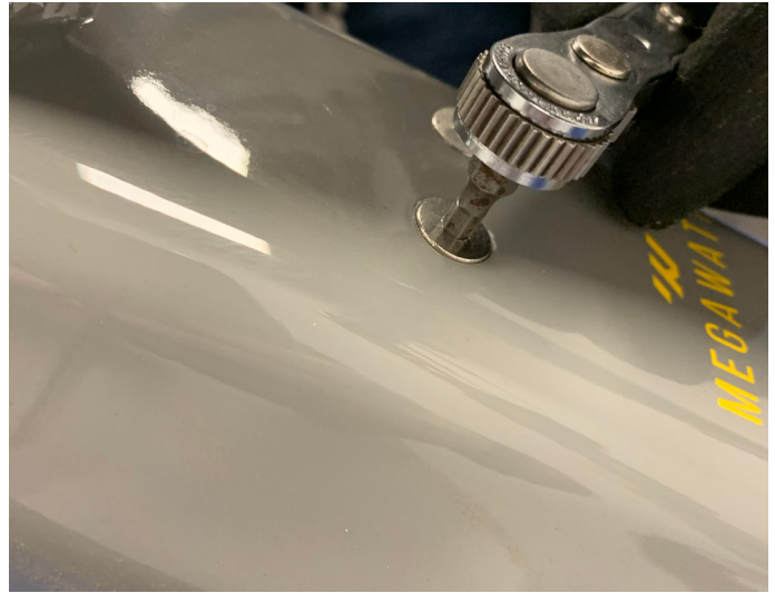
24. Remove 2x bolts of battery mount on outside of downtube
