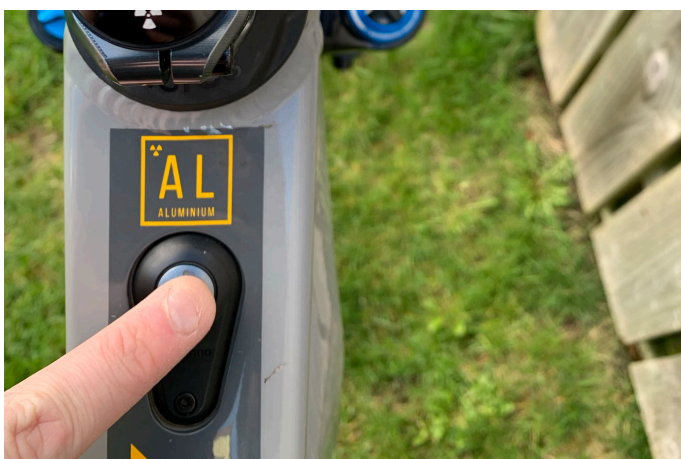
5. To switch off the bike at the end of the ride, press and hold the power switch until the screen goes blank
