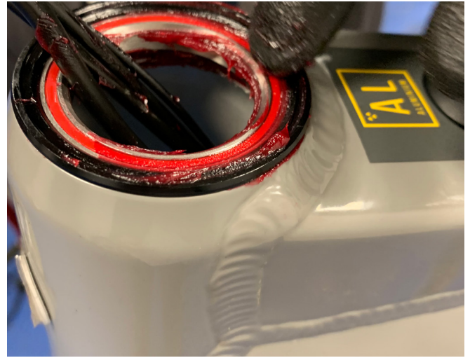
48. Apply grease to top of bearing
