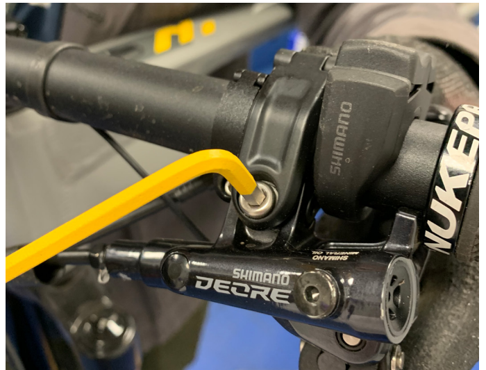
8. Move brake lever on the brake which has the hose routed via the headset to a flat position on the handlebars
