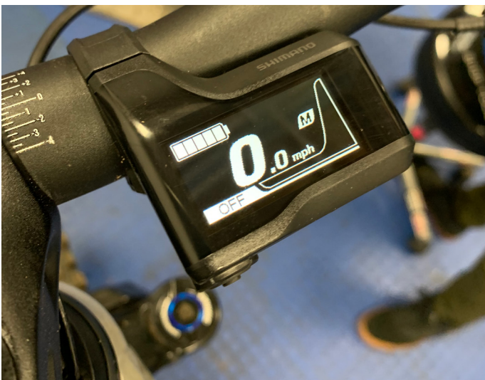
75. Switch on bike and ensure that it powers up and mode switch works as intended
