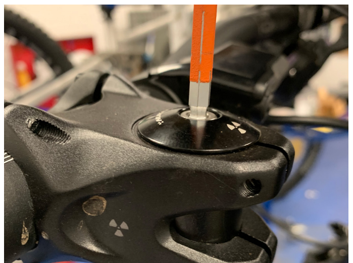
58. Fit top cap and lightly tighten bolt to hold fork in place
