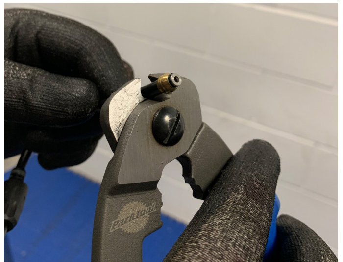
10. Cut old olive / insert and remove nut / rubber protector from brake hose
