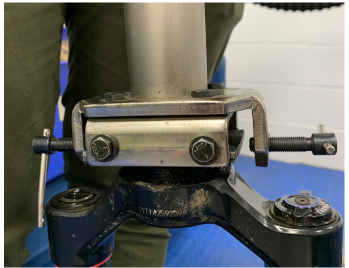
32. Get crown race removal tool and remove crown race from fork
