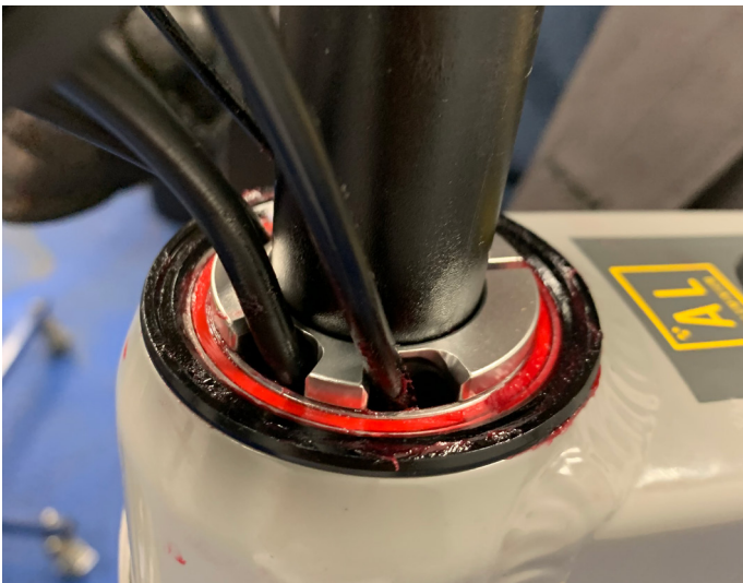
55. Insert compression ring and press into place with cables in correct slots
