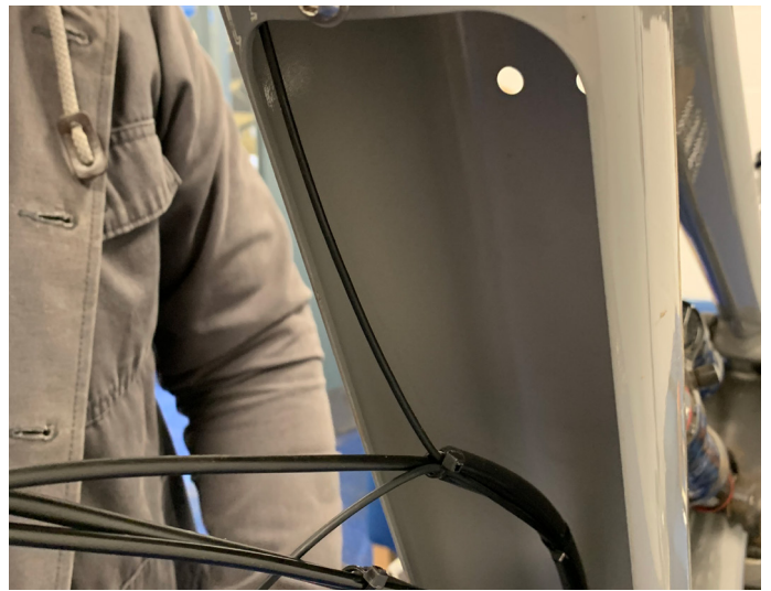
26. Carefully pull cables / hoses through the headset and out of downtube. Note: One cable will remain which is connected to the power switch on top tube and does not need removed
