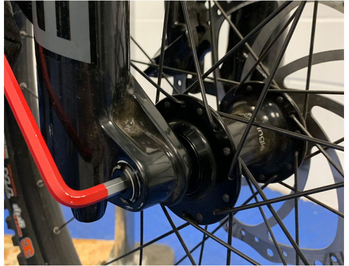
6. Remove front wheel from bike following fork manufacturer's instructions
