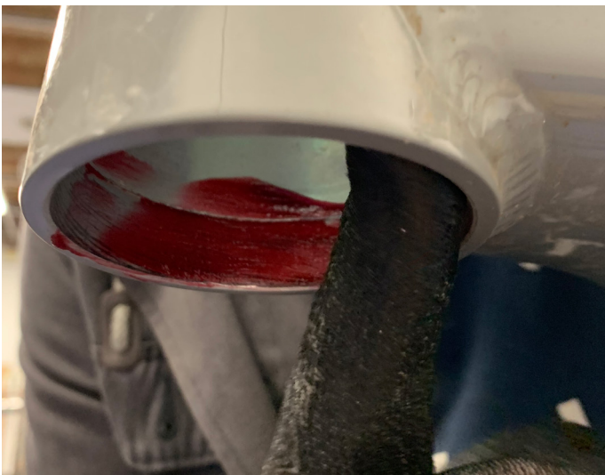
39. Apply grease to inside of the bottom of the headtube
