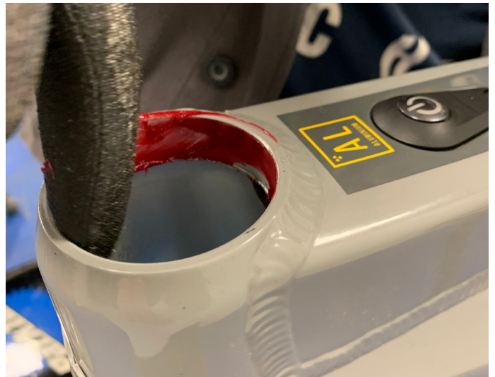
38. Apply grease to inside of the top of the headtube
