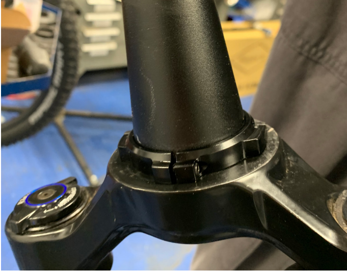
35. Place crown race on fork - bolt hole goes to front
