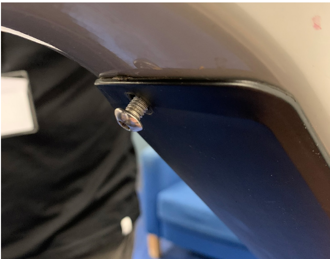
69. Refit battery door and tighten top bolt
