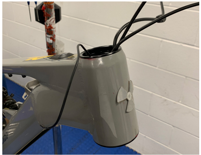
44. Feed cables back through the headset - be careful not to get cables tangled with the power switch cable which was not removed
