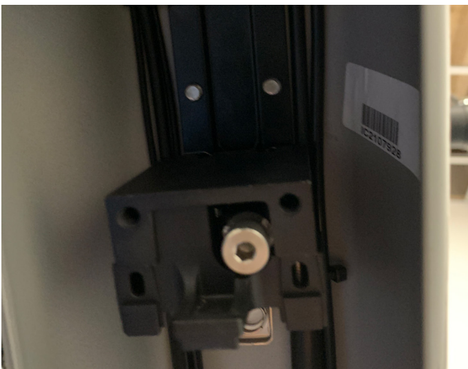
45. Refit battery mount / cable holder. Push cables into the holder and ensure that cables are not trapped under the mount before tightening the bolts on outside of downtube
