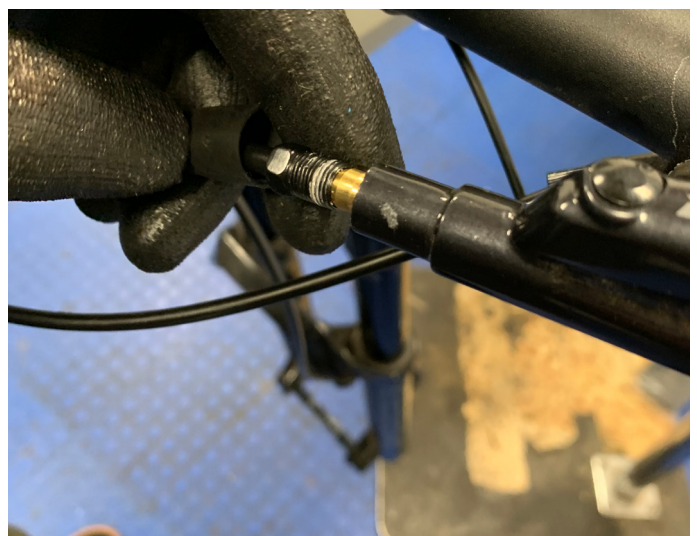
64. Reconnect brake hose by fitting new olive / insert. Follow manufacturers instructions for your specific brake
