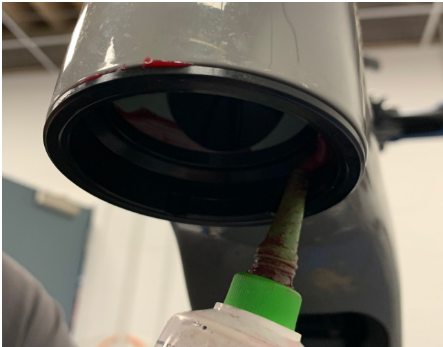
49. Apply grease to inside of bottom headset cup
