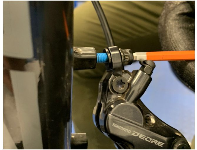
60. Refit front brake calliper and tighten bolts until calliper holds in place but can still be moved by hand
