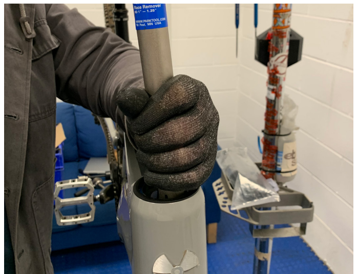
28. Insert headset removal tool for bottom cup
