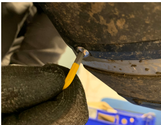
3. Loosen battery door bottom bolts 2 full turns
