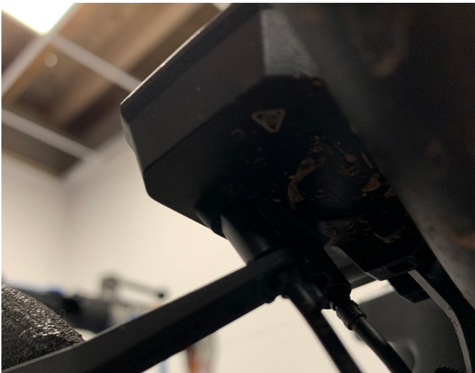
7. Disconnect di2 cables from screen using Shimano TL-EW300 tool
