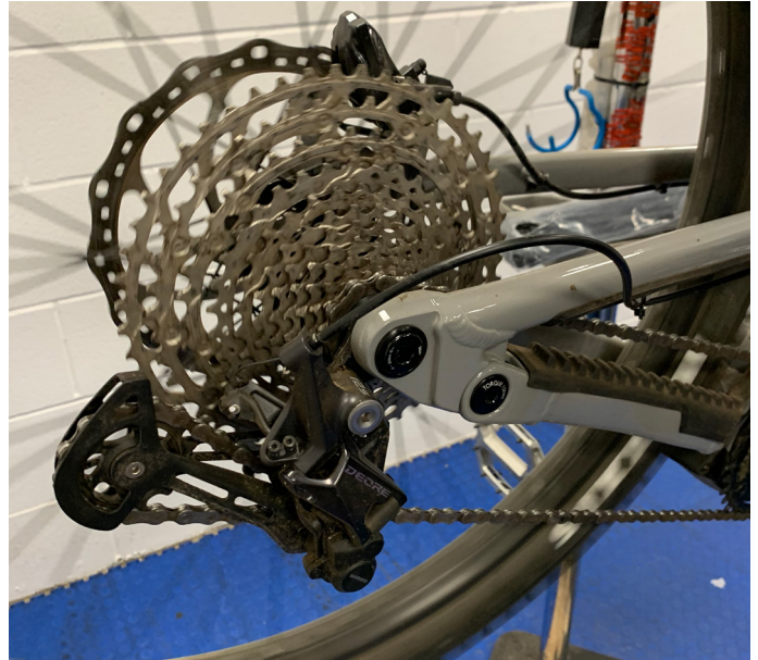
12. Spin cranks and shift chain to smallest sprocket
