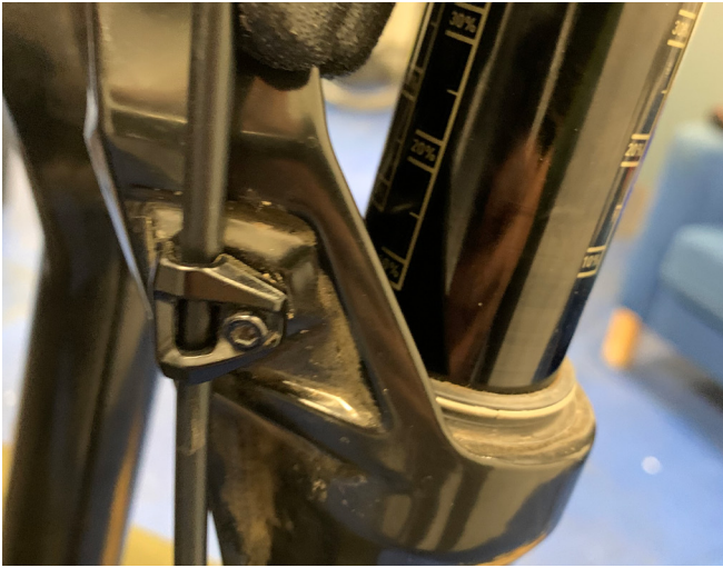
59. Refit fork cable hose guide to hose
