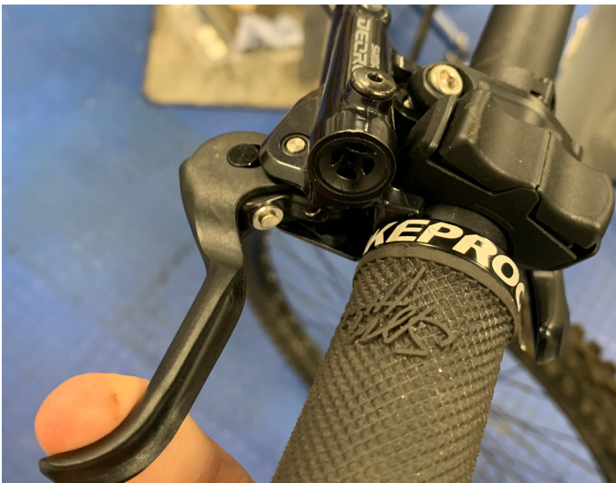
73. Check brake function and rebleed brake if needed following manufacturer instructions
