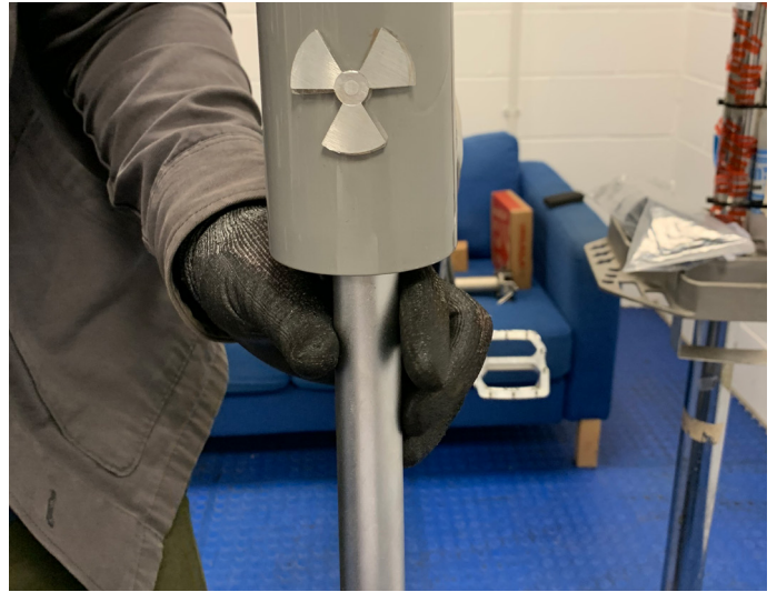
30. Insert headtube removal tool for top cup
