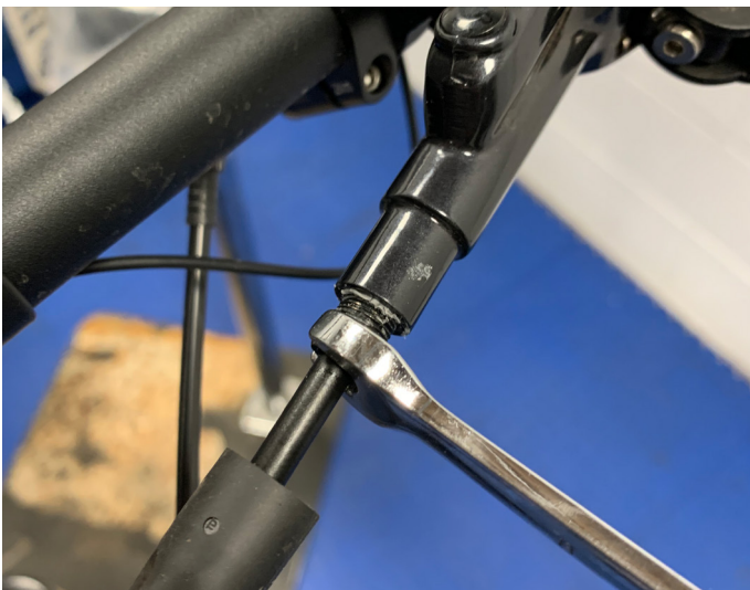
9. Disconnect brake hose (on brake which has hose routed via headset)
