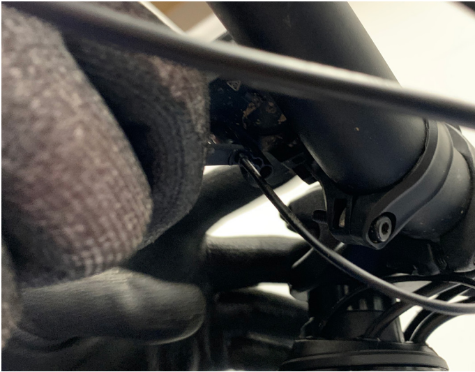
65. Reconnect di2 wires to screen using Shimano TL-EW300 tool
