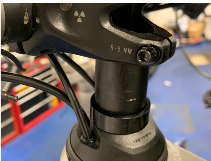
57. Refit stem and any headset spacers. There should be approx. 3mm gap between top of steerer tube and top spacer or stem to ensure headset can be adequately tightened. Your new headset may have a different stack height to the one you removed so different sizes of spacers may be needed.
