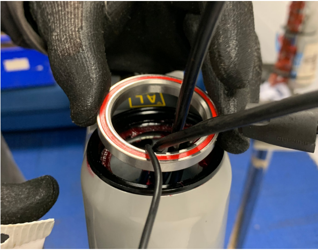
47. Insert top bearing (ensure chamfered edge on bearing is inside cup). The cables need fed through the centre of the bearing
