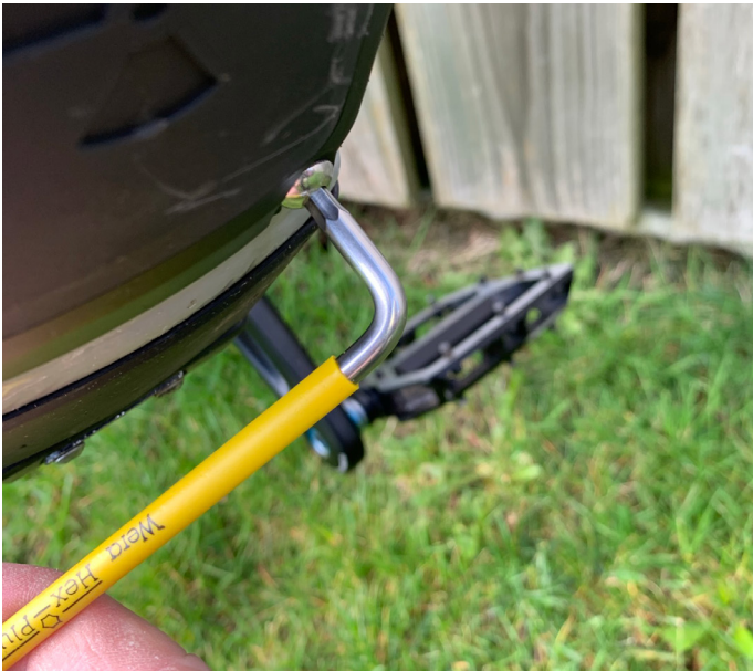
17. Tighten the lower right bolt using your 4mm hex key
