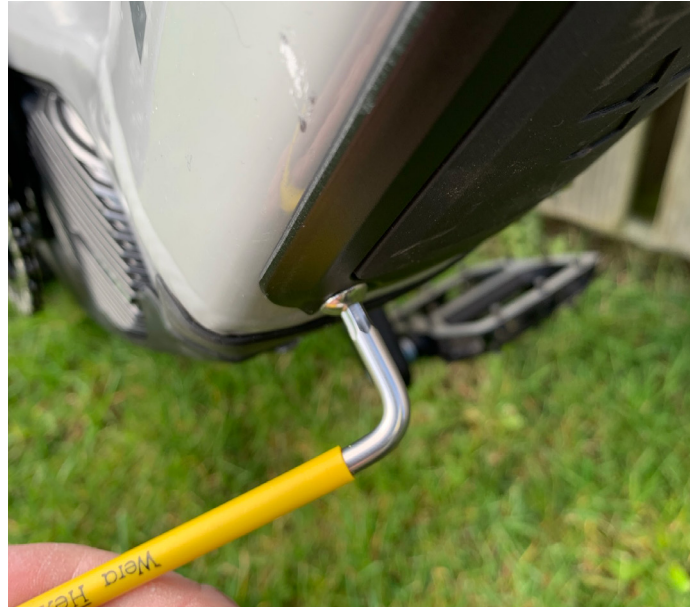
16. Tighten the lower left bolt using your 4mm hex key
