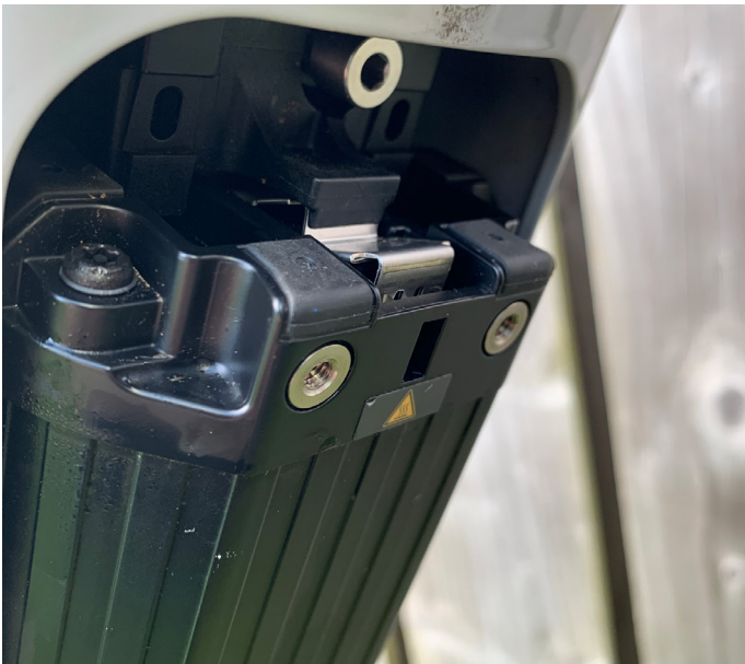
7. The battery should slide forwards and stop as per photo
