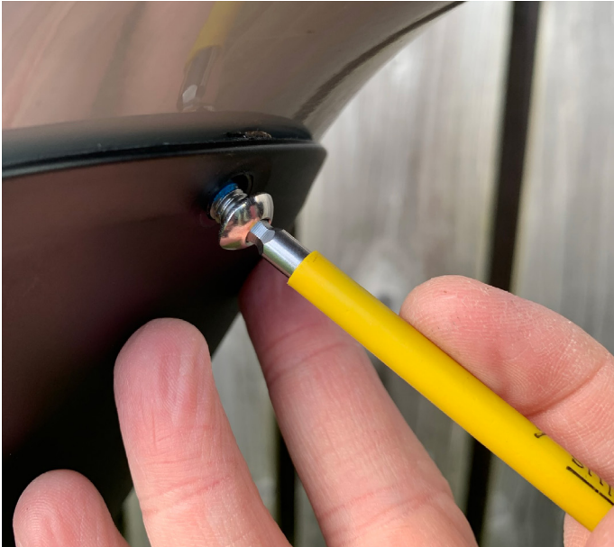
15. Tighten the top bolt first using your 4mm hex key
