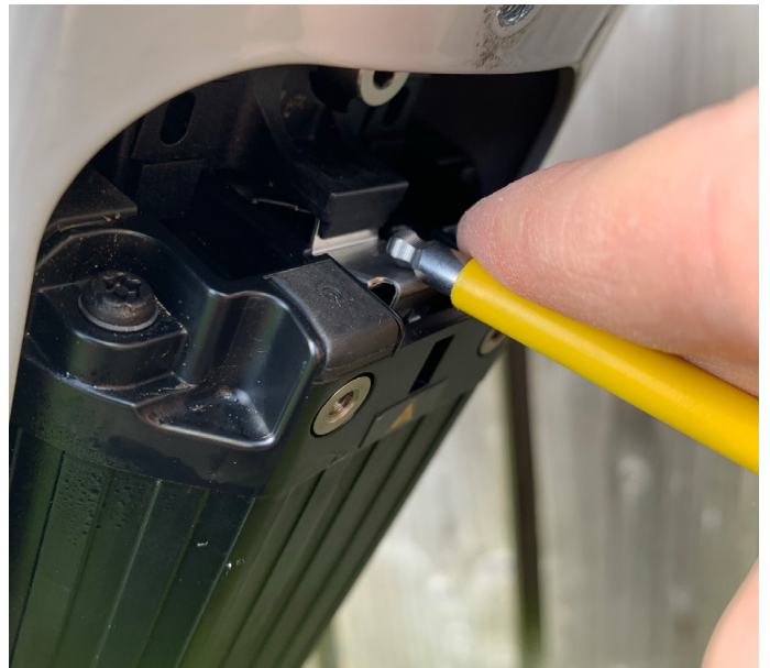
8. Push the silver clip down to fully release the battery
