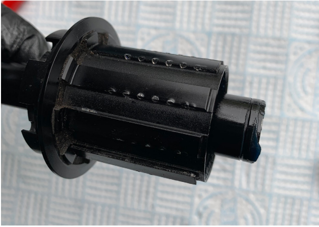
9. With the bearings now in place, take your axle and push it through the freehub to ensure the spacer is now fully central and the axle goes through correctly.
