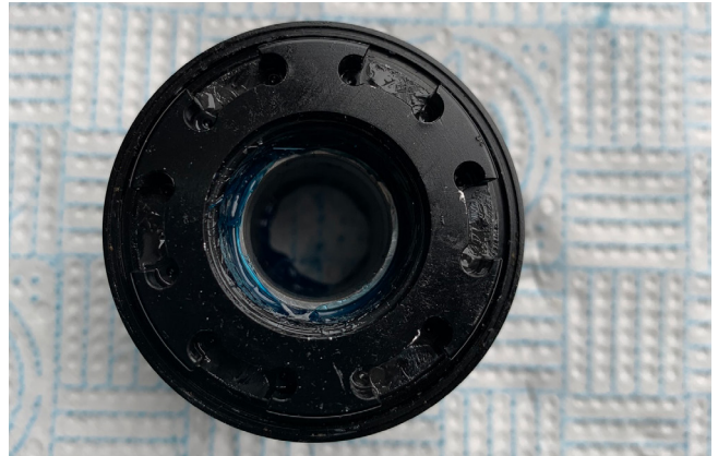
12. Turn the freehub over so the rear of the freehub can be seen.
