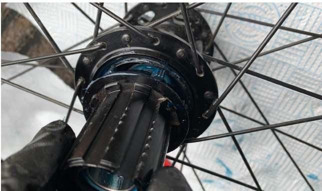
29. Slot the freehub over the axle, push onto the hub turning ANTICLOCKWISE as you do this to prevent damage to the seal.
