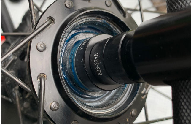
19. Press the bearing into the shell. Ensure it spins smoothly.
