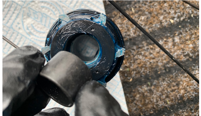
28. Refit the freehub spacer into the rear of the freehub.
