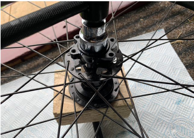
21. Take your non-driveside bearing and press it into place. On this we have used the block of wood to allow the axle to "float" and for the press to then push against the hub shell to allow the non-driveside bearing to be pushed into place.
