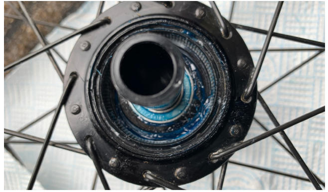
26. Apply a layer of grease to the ratchet ring and around the driveside bearing in the hub shell.
