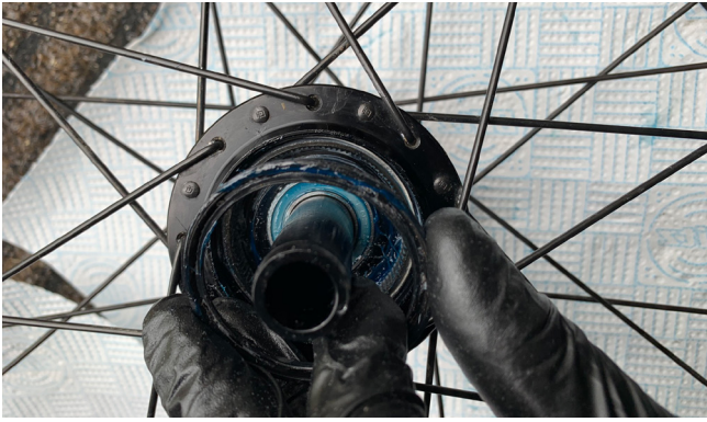
25. Apply a layer of grease to the hub shell freehub seal and push onto hub shell.
