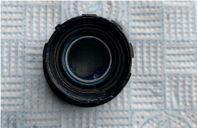
11. Reinstall the driveside freehub seal.
