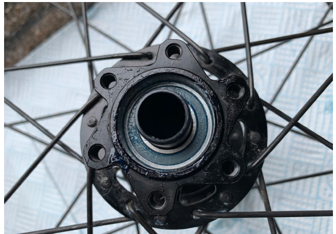
22. Apply a layer of grease to the non-driveside bearing.
