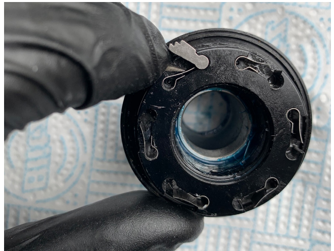
14. Refit pawls – you will need to use the flat head screwdriver to push the springs down to allow you to get them in.
