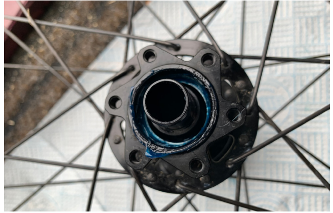
20. Put the axle into the hub through the non-driveside.
