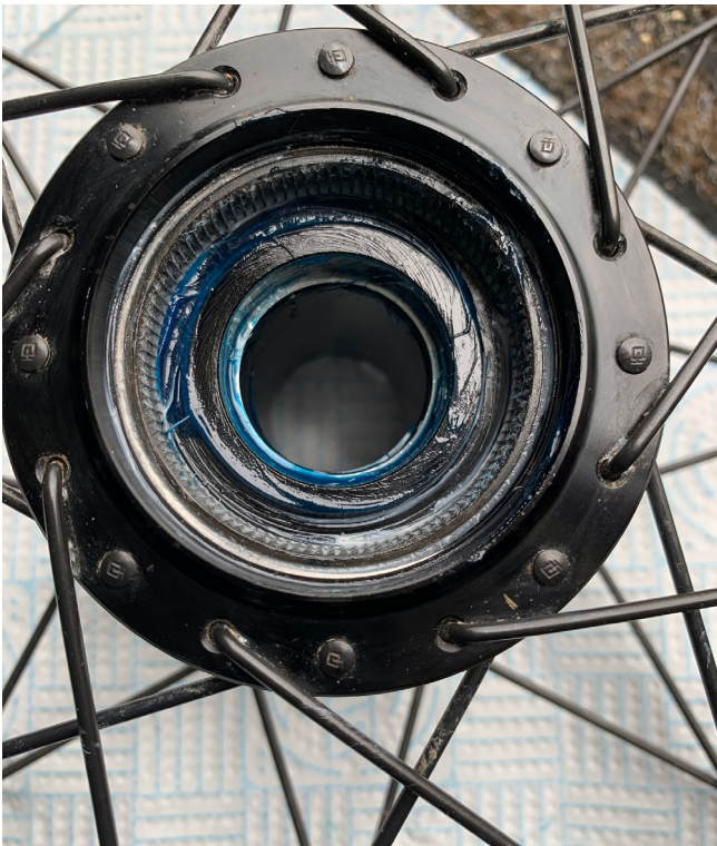
17. Check both sizes of the shell where your bearings will be pressed are smooth and free from burrs then apply a layer of grease.
