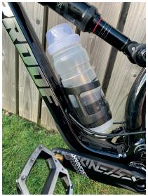
5. Insert water bottle and check it can be inserted & removed. Also ensure cage is tight.
