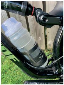
6. On a full suspension frame, it can be worth "bottoming out" the shock to ensure that the cage or bottle is not in the way as the framegoes through its travel.
