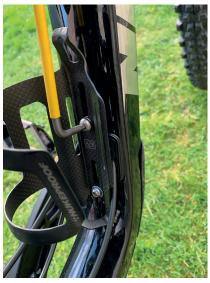
4. Slide the cage to the desired position and tighten bolts. Your Nukeproof cage has 40mm of adjustment.
