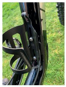
3. Put the bottle cage on your frame and insert both bolts.
