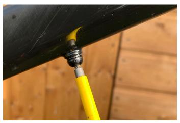
3. Use a 3mm hex key to remove the bolts on the underside of the top tube.
