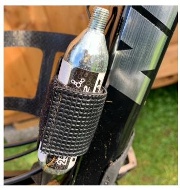
9. Get a 25g co2 cartridge and tighten in the strap. This could also be used to carry a small diameter pump.
