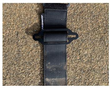
Thread the strap through the backplate. Note: The rubber side should be facing the same way as the Nukeproof logo on the backplate.
