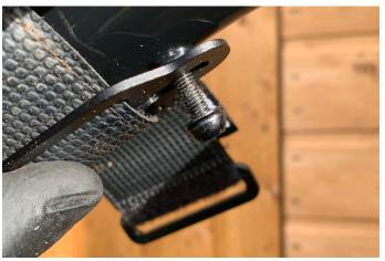
4. Put the plate up to the frame and then reinsert bolts.
